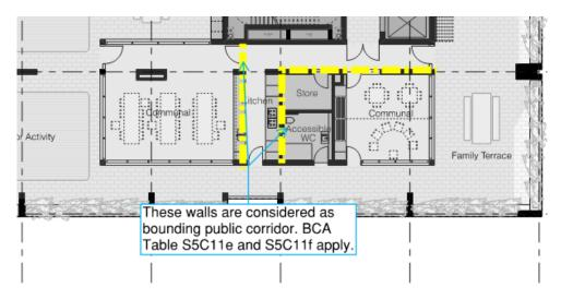
Similarly at S3, the residential corridors are generally considered to be open balcony between Ground to Level 4. However, at Level 5 to 6, requirements of C4D12(9) as the south apartments are provided with single path of travel only. At Levels 7 to 9, the corridor not considered as open balcony, and requirements of Table S5C11e and S5C11f apply.
