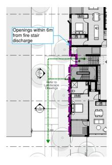
• S3 north and south fire stairs at north and south elevations facing the internal courtyard
