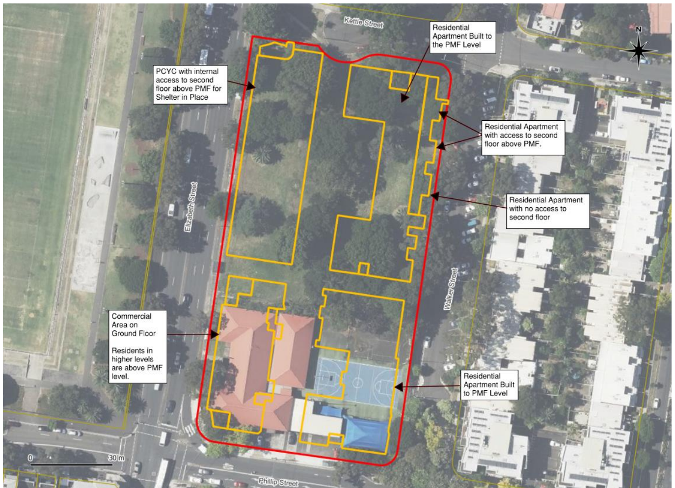
Figure 5-5: Building Access to Areas Above the PMF Level
