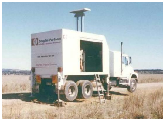
Figure 2: Purpose built CPT rig
