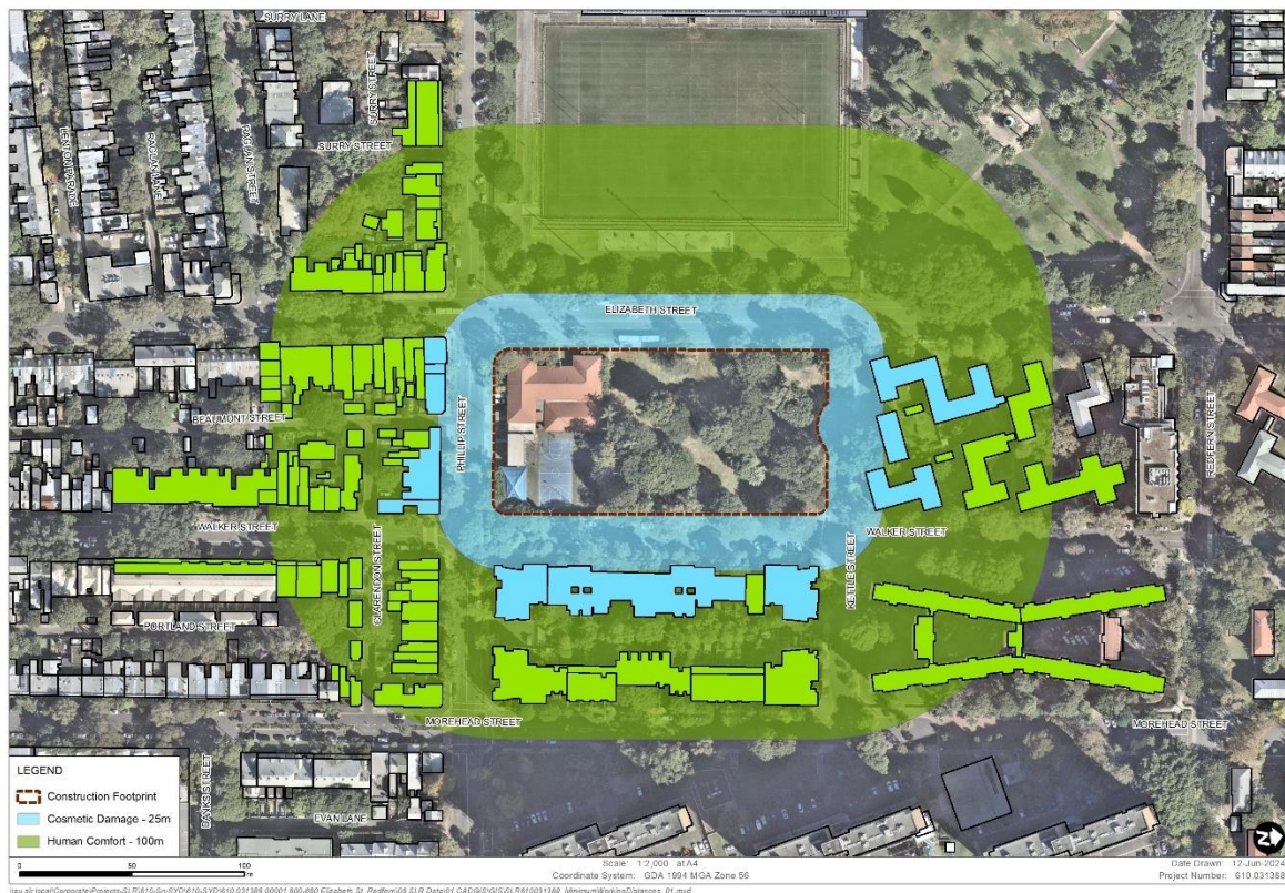
Figure 11 Construction Vibration – Large Vibratory Roller
