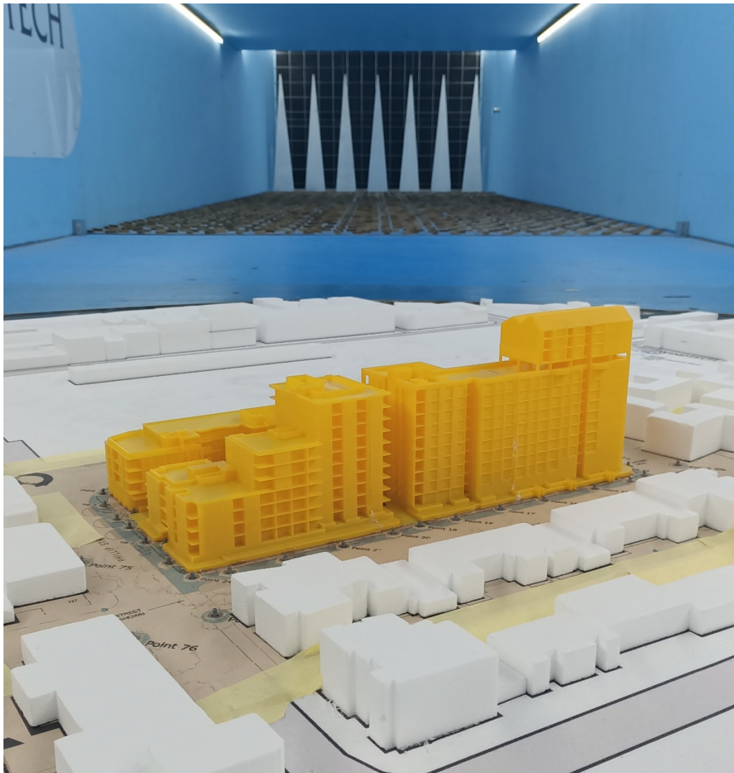
Figure 1a: Photograph of the Wind Tunnel Model (proposed scenario, view from the south-east)
