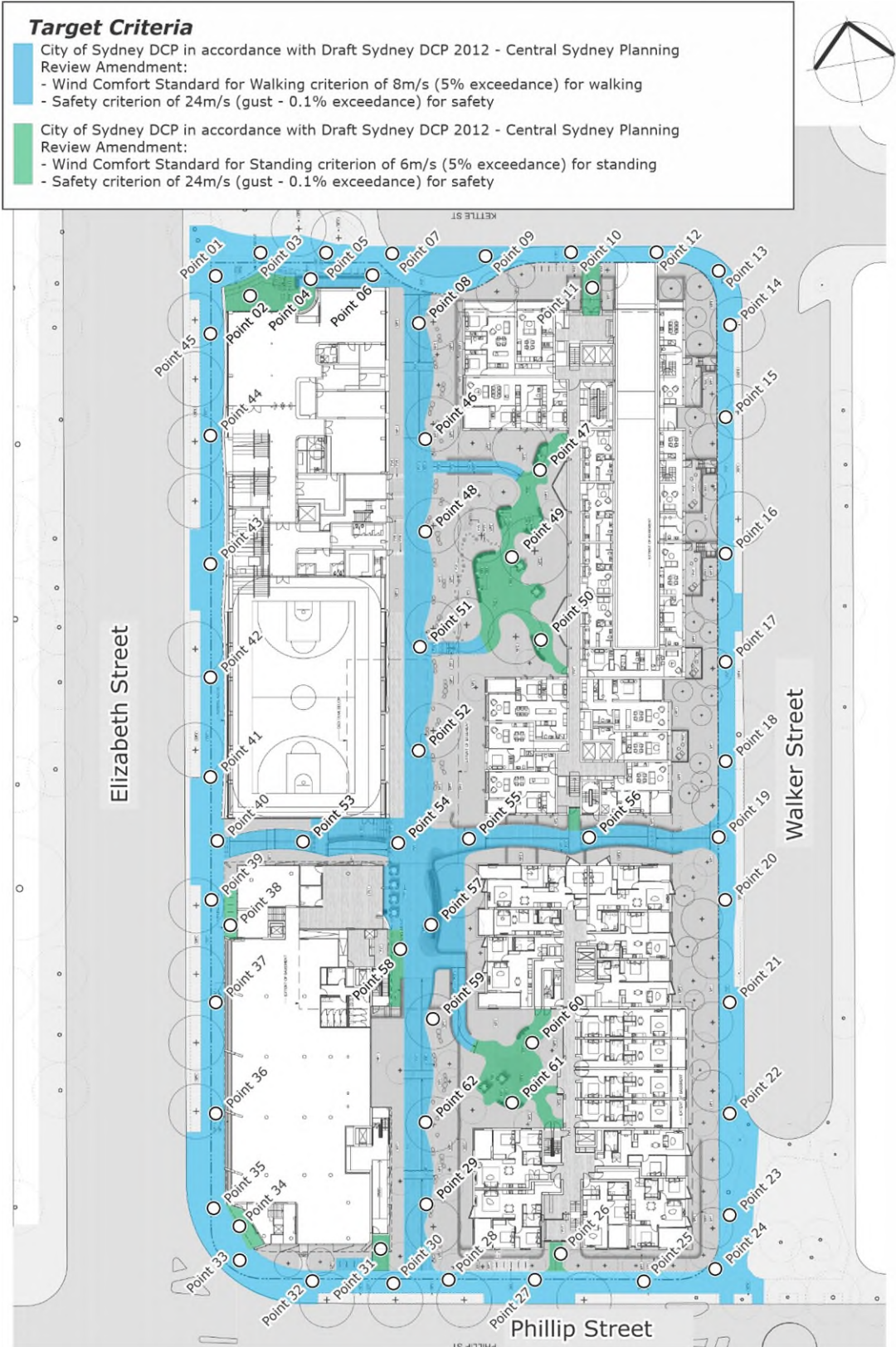
Figure 5a: Study Point Locations and Target Wind Speed Criteria – Ground Floor Plan
