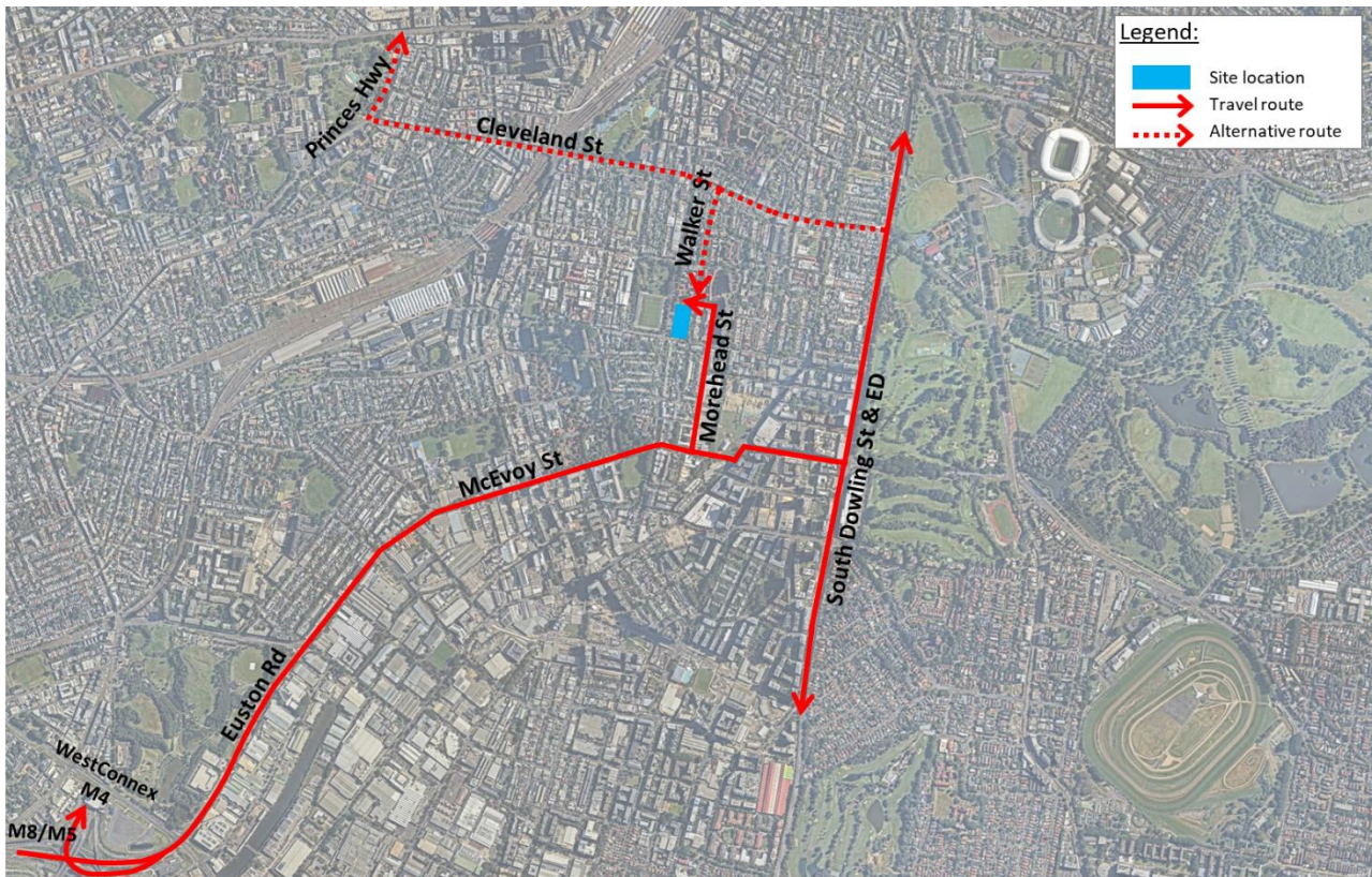
Figure 17: Anticipated Construction vehicle routes
