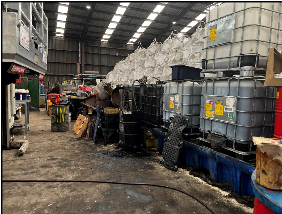
Photo 5: Flammable liquids cabinet and an IBC on a pallet bund near the southern entrance to the Shed D Workshop. Oil spill on the floor around the bund.
