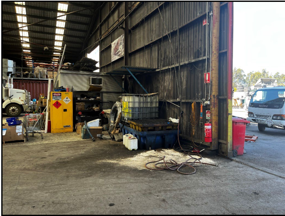
Photo 5: Flammable liquids cabinet and an IBC on a pallet bund near the southern entrance to the Shed D Workshop. Oil spill on the floor around the bund.
