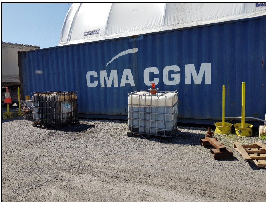
Photo 18: Unbundled IBCs next to the AN unloading shelter. Collected AN prill is emptied into the IBC containing water on the right.
