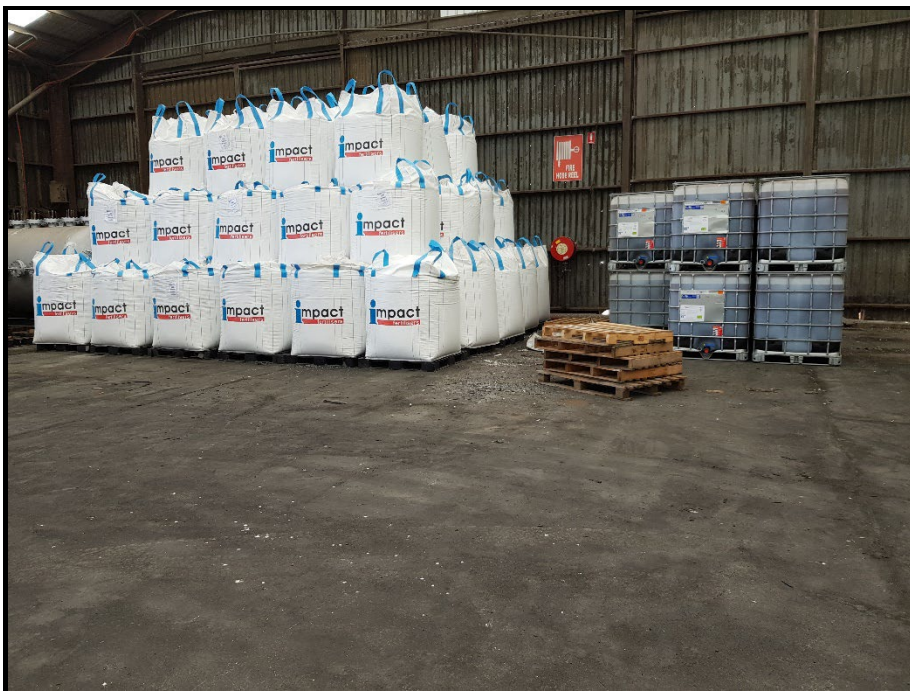
Photo 2: Chemical storage within northern half of Shed D, north-eastern wall. Unbundled IBCs. Restricted access to fire hose reel.
