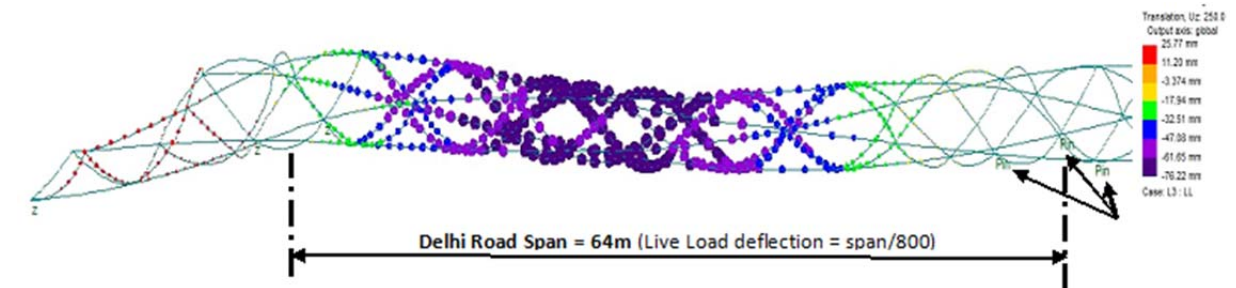
Figure 14: Vertical serviceability displacements under trunk services and LL
