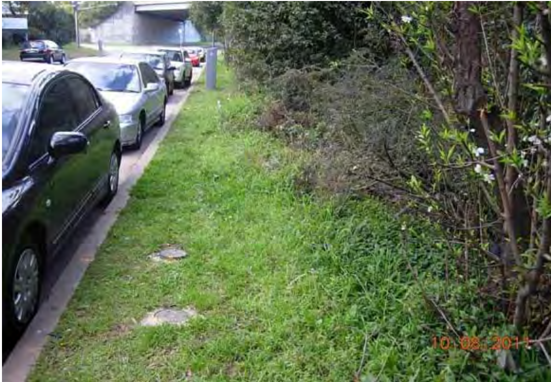
Photo 19 (August 2011) - Two of the groundwater wells observed near northern boundary
