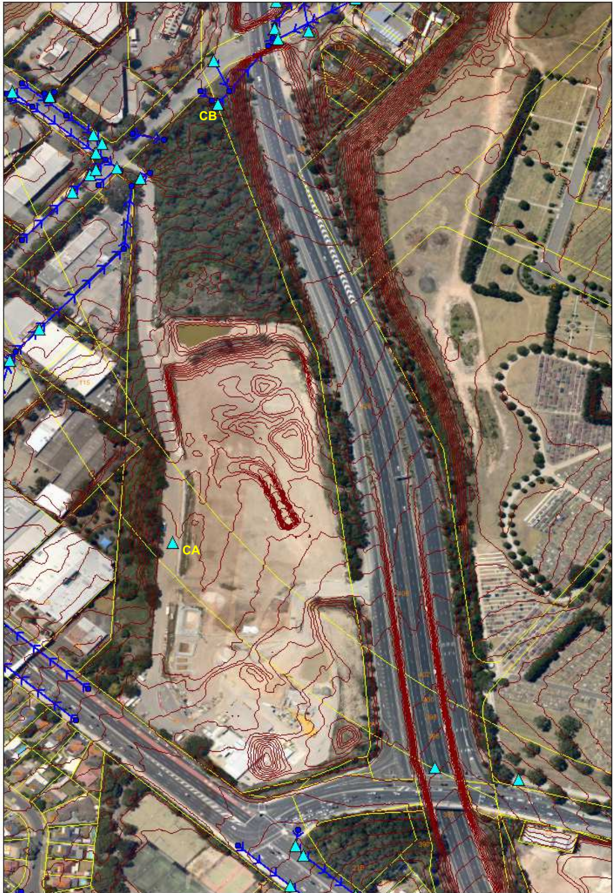
Figure 12 Location of Inflows (Blue Triangles) in Council's Porters Creek TUFLOW Model
