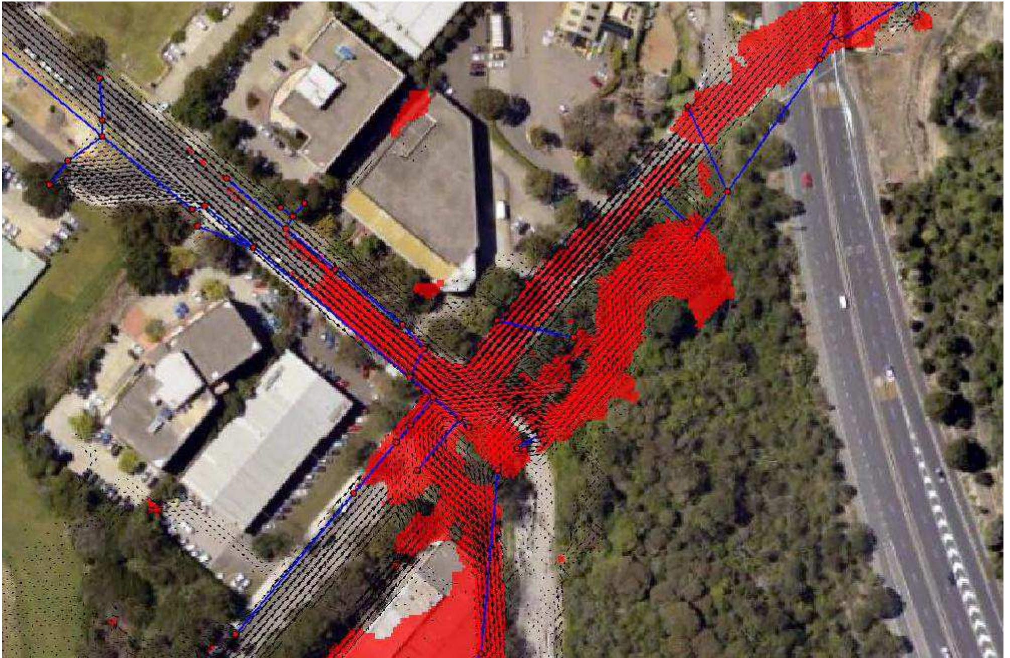
Figure 6 100 yr ARI Flood Velocity Vectors – Benchmark Conditions
