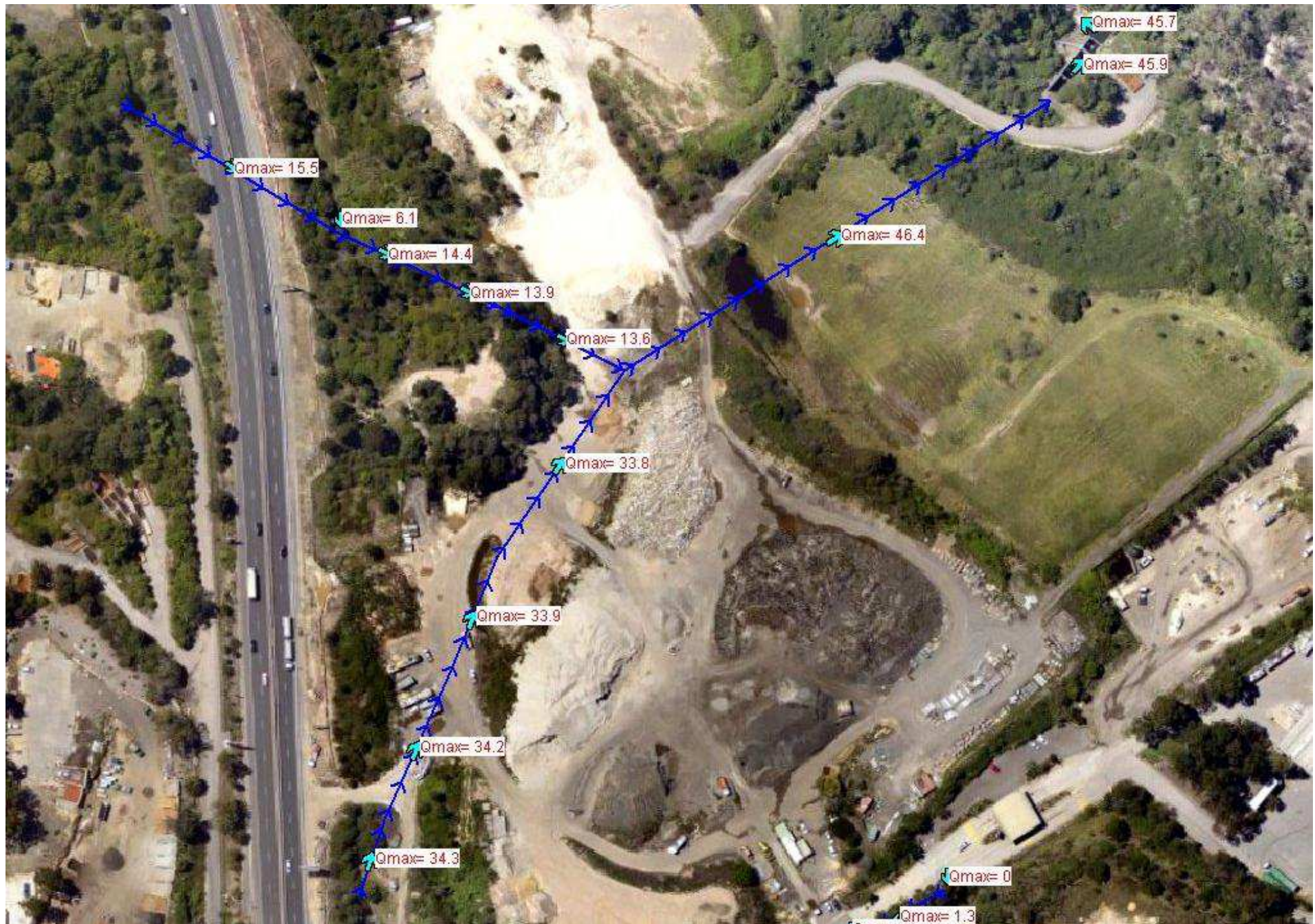
Figure 8 100 yr ARI Peak Flows in Downstream Drainage System – Benchmark Conditions
