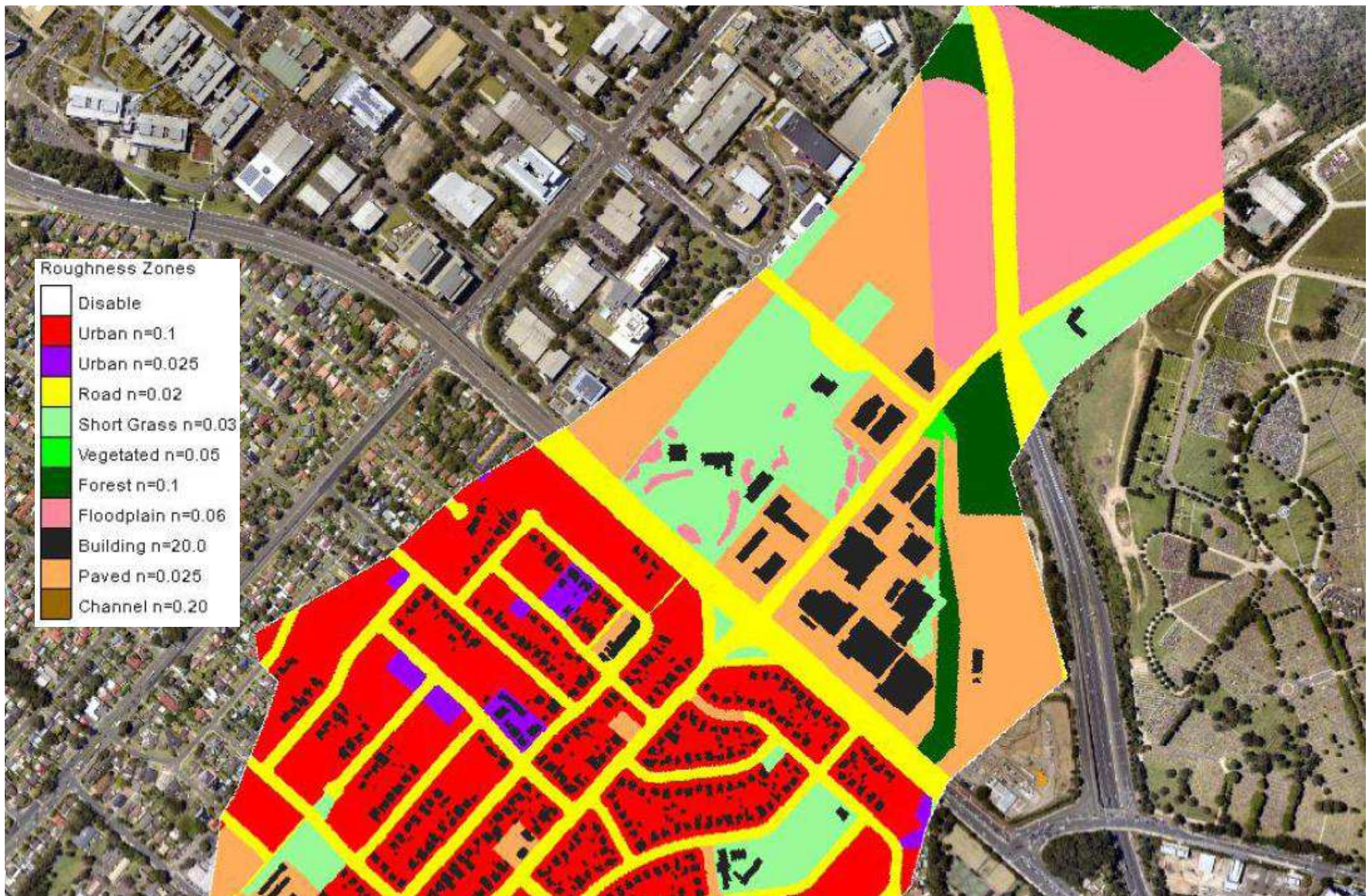
Figure 5 Adopted Roughness Zones – Benchmark Conditions
