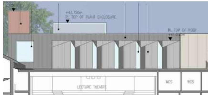
Figure: South facing skylights would harvest diffused daylight.
