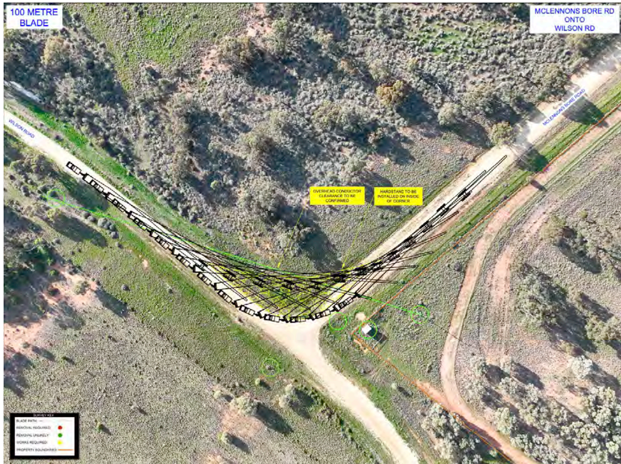
Figure 33 - Mclennons Bore Rd onto Wilsons Rd
