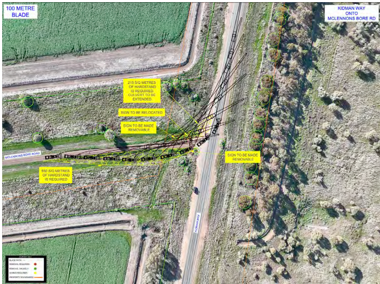
Figure 32 - Kidman Way onto Mclennons Bore Rd
