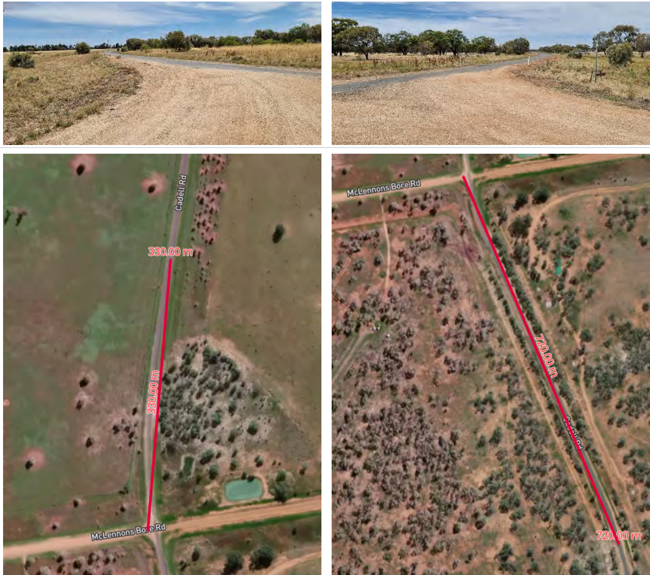
Sight distance to the left from McLennons Bore Road west approach (330 m)
