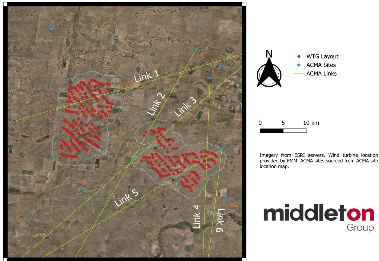
Figure 1: Wind turbine layout overlaid with telecommunication services
