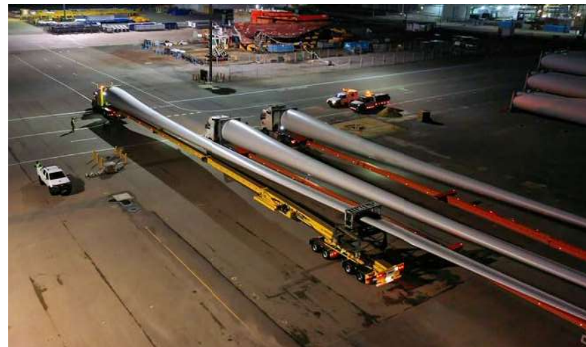
Above: 75m-long blades loaded on extendable blade trailers for the Yandin Wind Farm project
