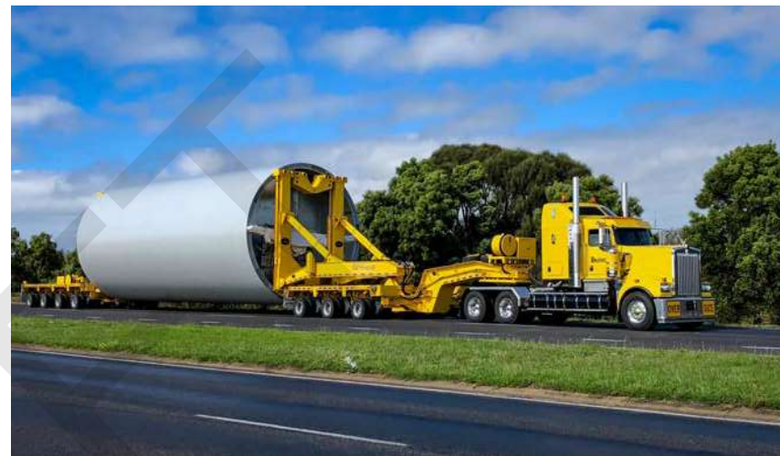
Above: Bookend Trailers being used by ARES for Murra Warra's 5.8m towers
