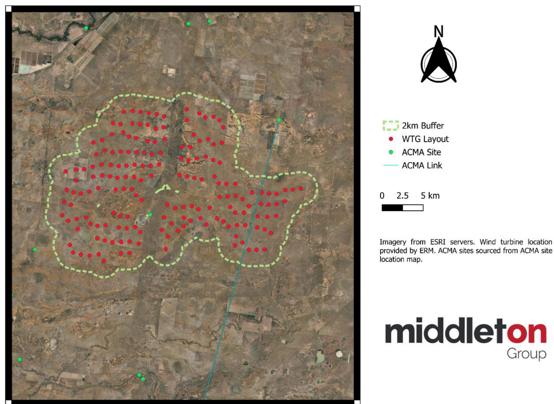
Figure 1: WTGs, 2 km buffer with ACMA communication sites and link assignments
