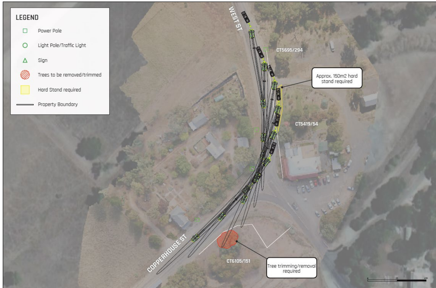
FIGURE 1.3 WORKS REQUIRED AT PINCH POINT 8, THE LEFT TURN AT COPPER HOUSE STREET AND WEST STREET, BURRA (ARES GROUP 2024: 50-51)
