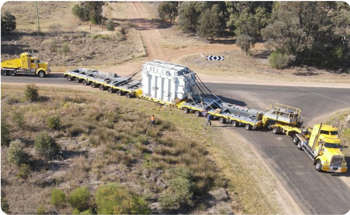
Above: ARES transporting a 170-ton transformer on a custom drop frame trailer. Below: Schematic of proposed trailer for Panorama BESS.
