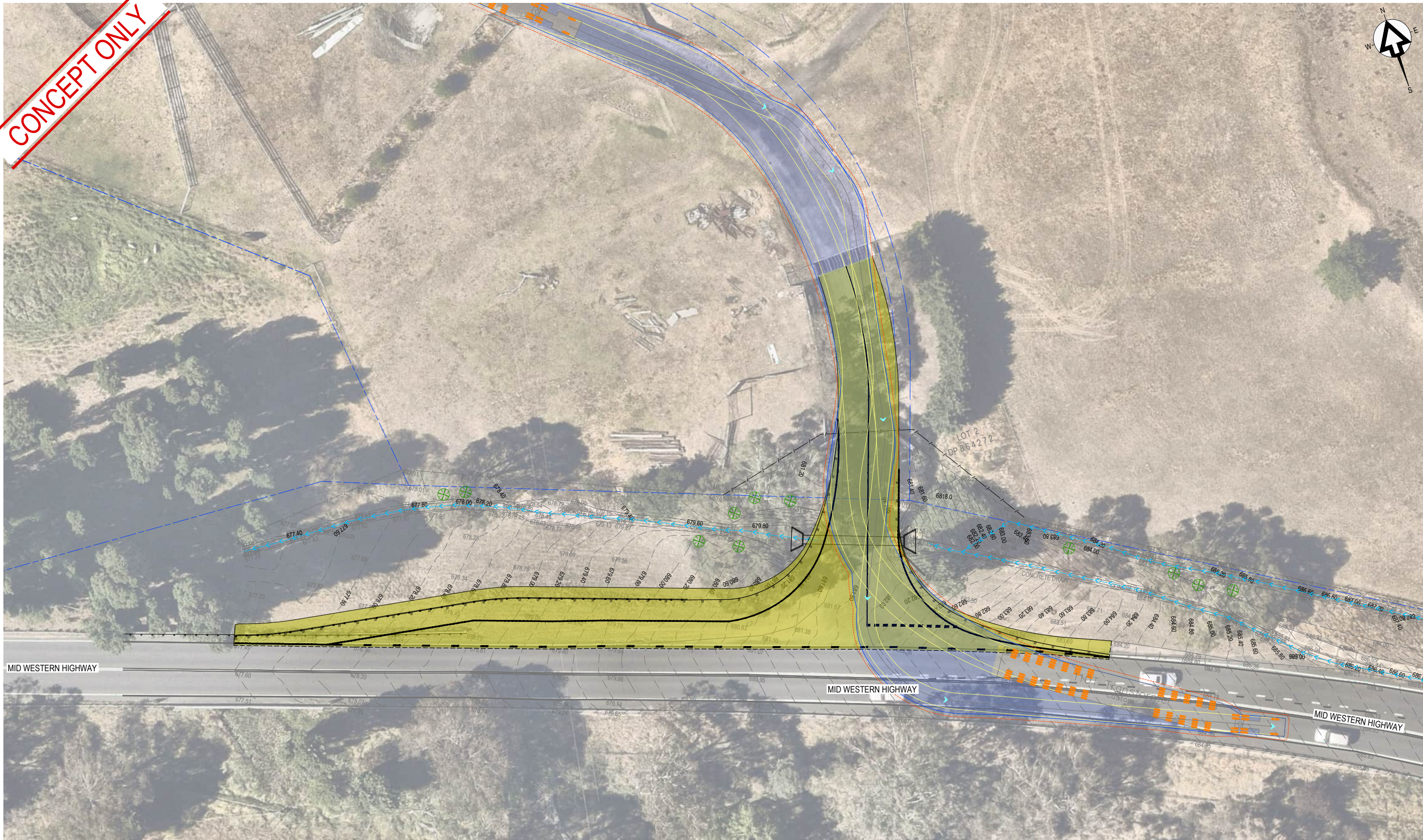
SWEPT PATH ANALYSIS - 100T TRANSFORMER EXITING PROPERTY ACCESS SCALE 1:250
