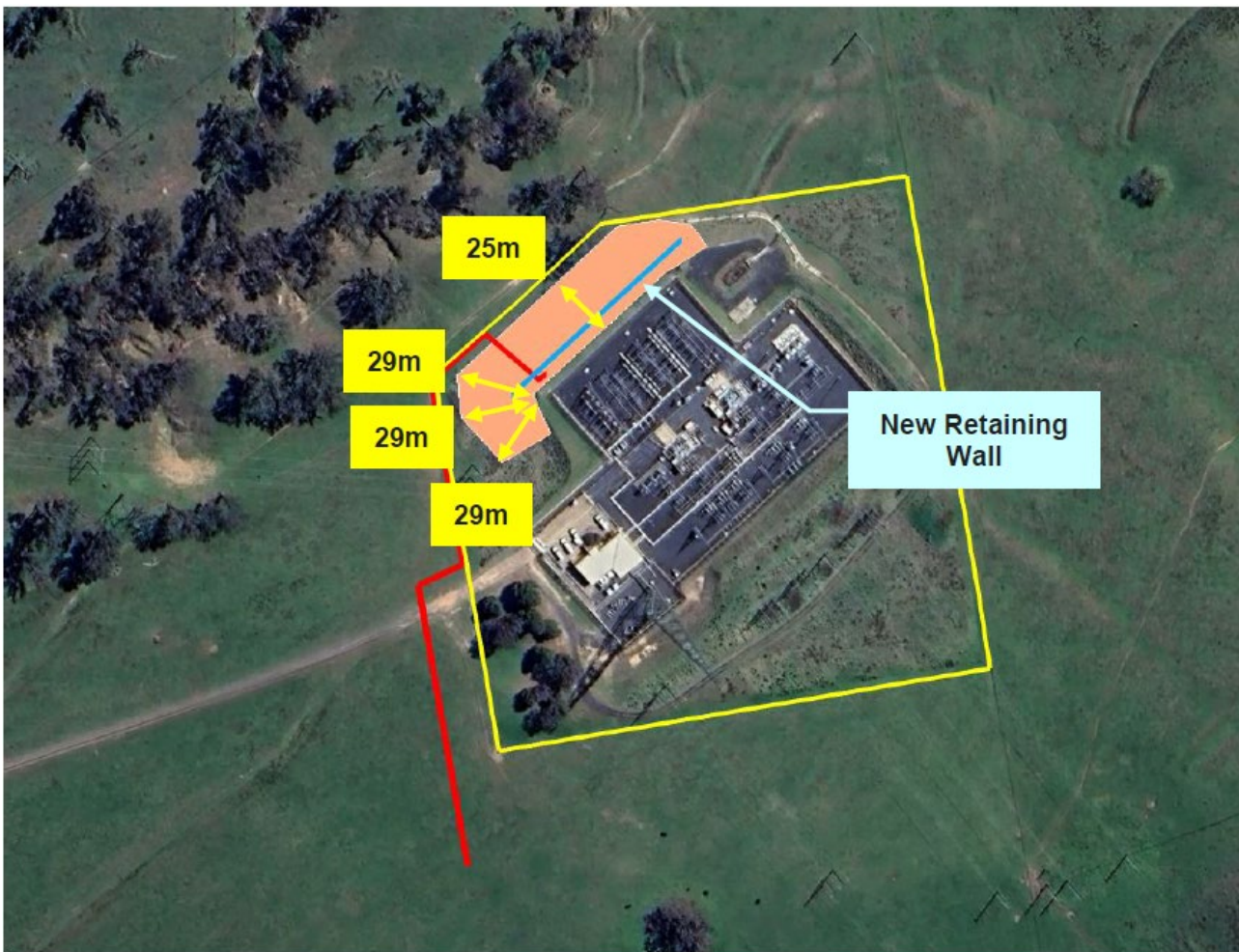
Figure 6-8 Transgrid Substation APZ (Source: SLR, 2026)
