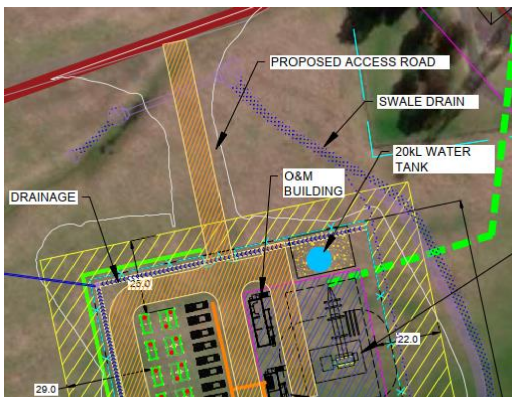
Figure 15 Dedicated Firefighting Water Supply
