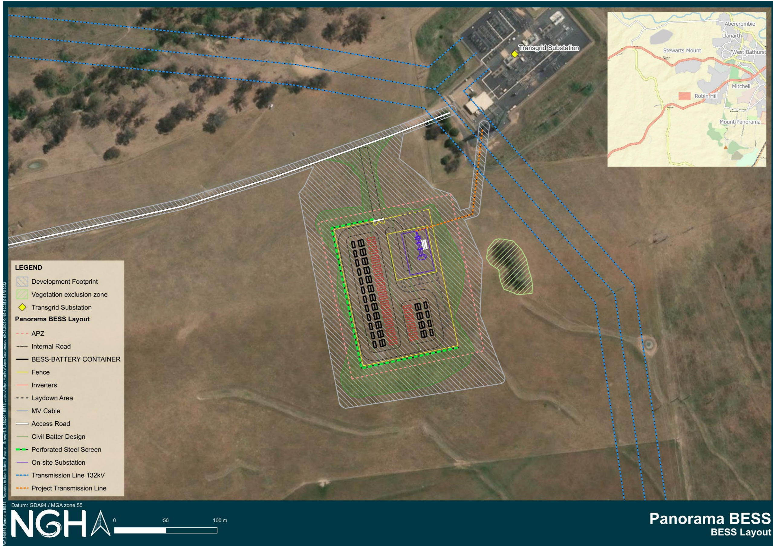
Figure A1-1 Panorama BESS Indicative Infrastructure Layout
