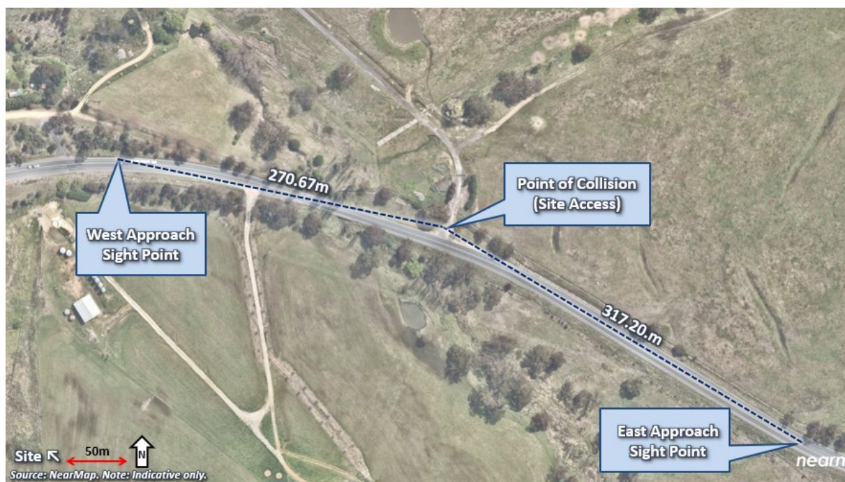
Figure 20: Access Location and Relevant Sight Distances
