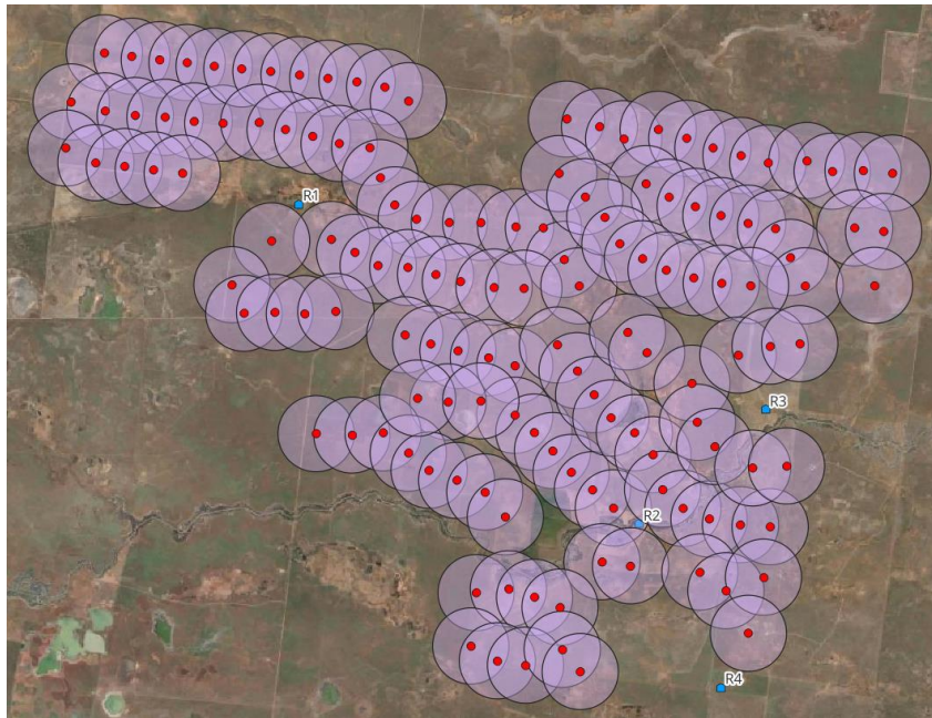
Figure 2a: Dwellings relative to fragment range (purple) of Original EIS candidate turbine
