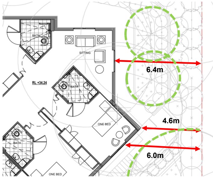
Figure 19: Building B - Setbacks eastern boundary (detail)
