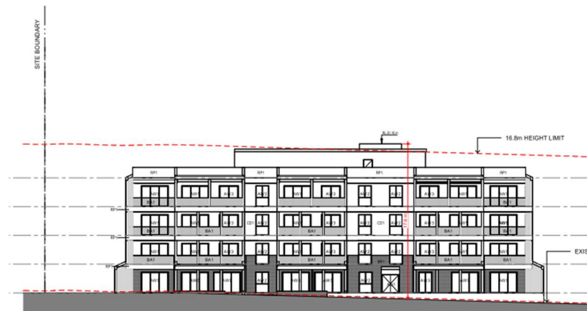
Figure 40: Extract Building E - west elevation
