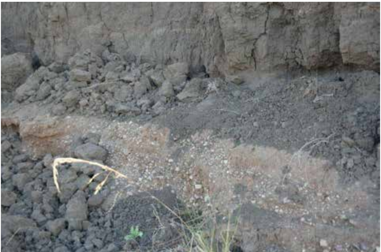
Figure 7.25: Soil Profile at Perfremment Road Crossing Showing Black Soils Overlying Sands and Gravels (265856 mE, 6549162 mN)
