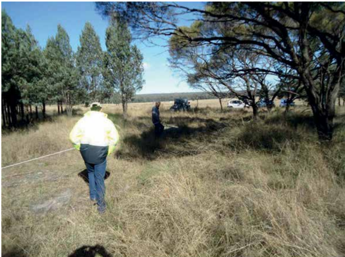
Photo 2: Running out the 100m tape at WM GG1 - 11 to establish the baseline.
