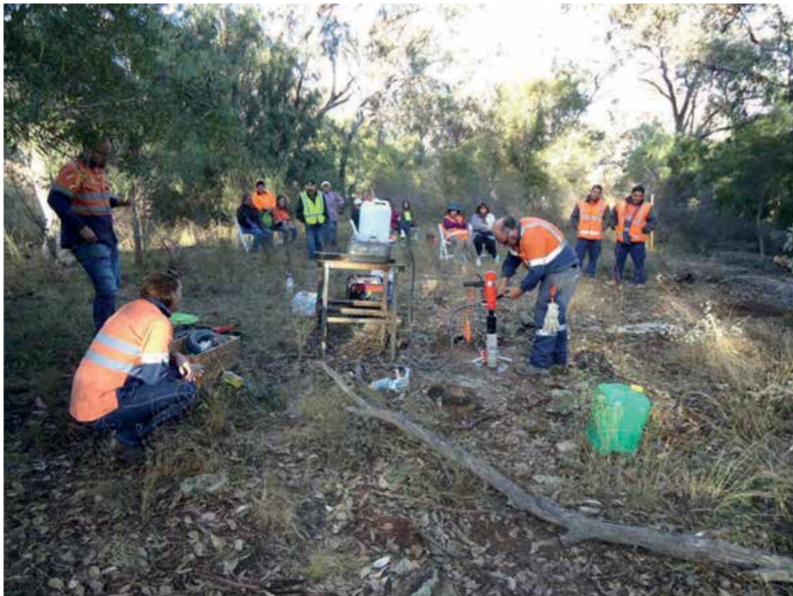
Photo 21: Core drilling the bedrock at WM GG3 - 12 and the Senior Elders Group.
