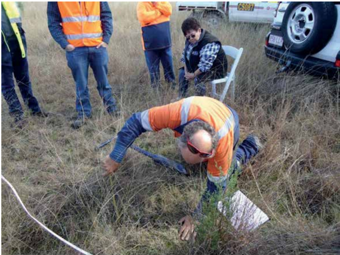
Photo 4: Engineering geologist Luc Daigle measuring the depth of an auger hole at WM GG1 - 11.
