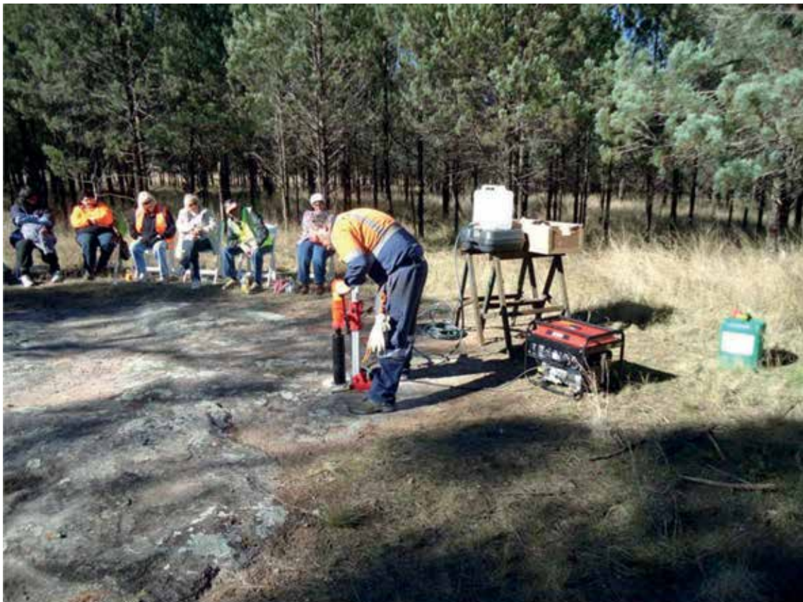
Photo 9: Hand coring the outcrop slab at WM GG1 - 11.
