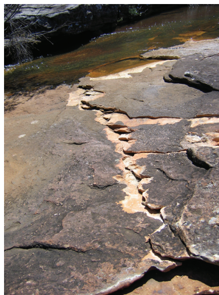
Fig. 4.13 Example of Sandstone Fracturing and Bedding Plane Slippage in Bedrock in the Base of a Stream in the Southern Coalfield
