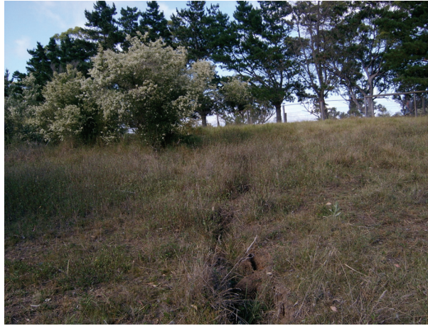
Fig. 4.11 Example of Surface Tension Cracking along the Top of a Steep Slope
