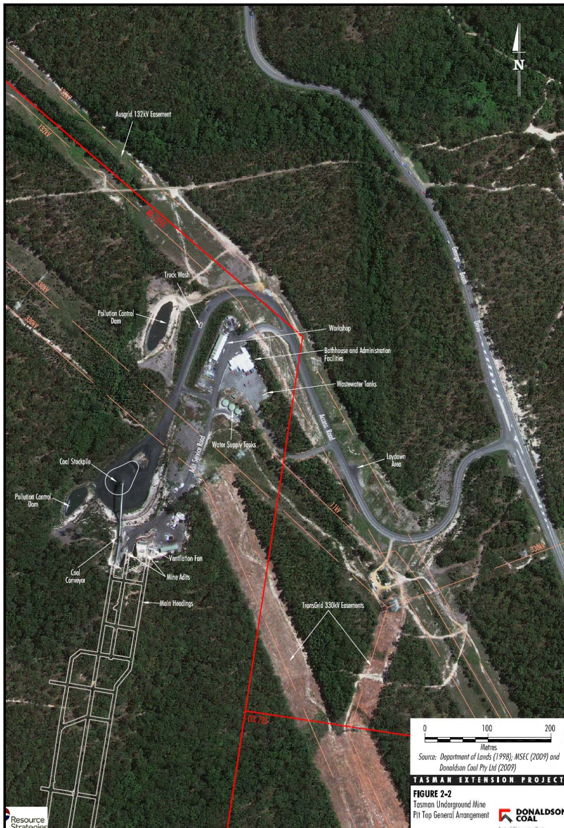
Figure 1: General Arrangement of the Existing Pit-Top site
