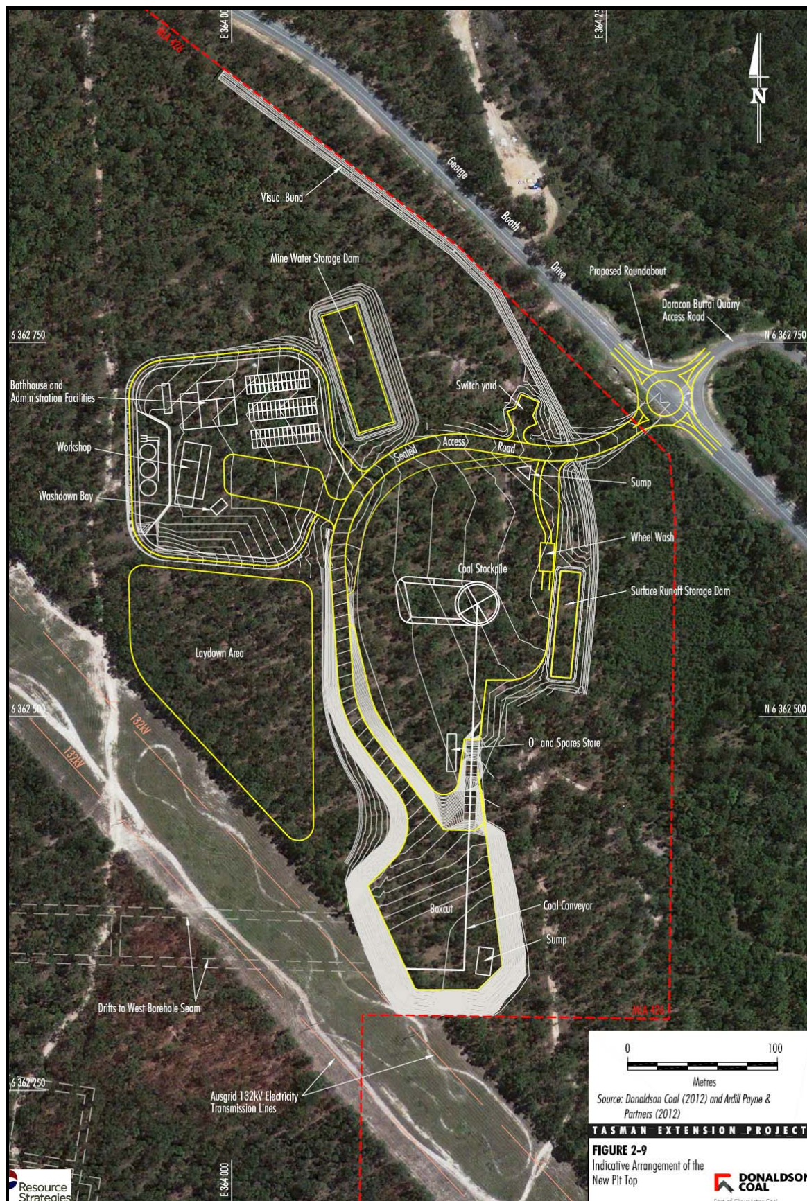
Figure 2: General Arrangement of the New Pit-Top site
