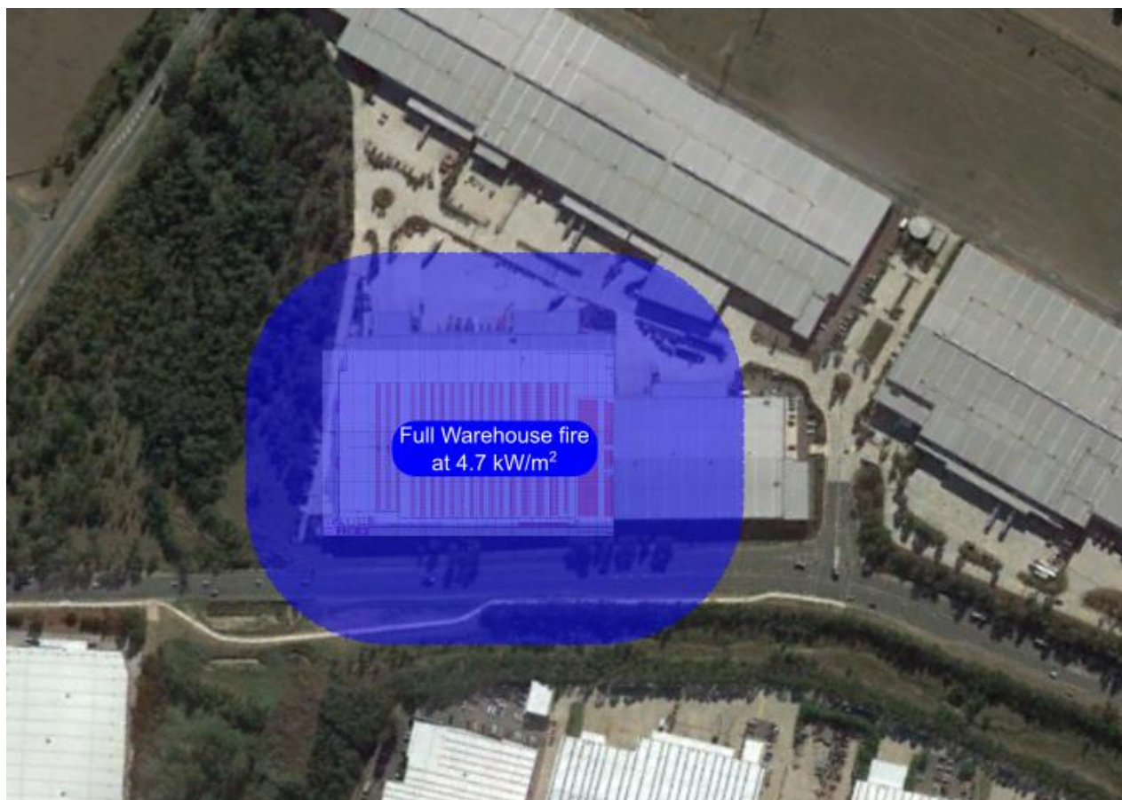
Figure 5-3: Full Warehouse Fire Radiant Heat Contours
