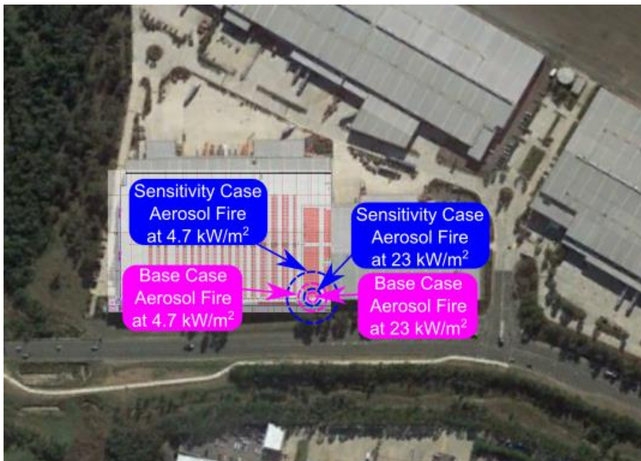
Figure 5-1: Sprinkler Controlled Aerosol Fire Radiant Heat Contours
