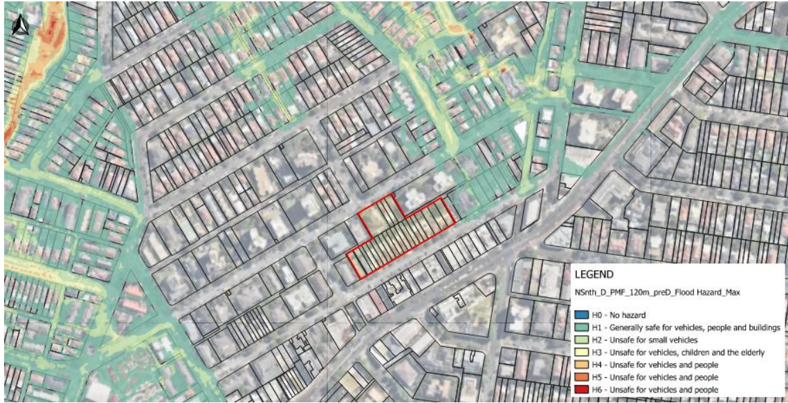
Figure 18 – Maximum flood hazard for 2-hour duration rainfall – PMF (pre-developed conditions)
