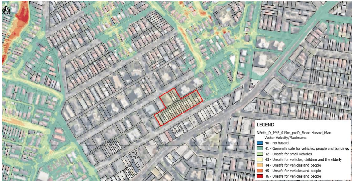
Figure 12 – Maximum flood hazard for 15 minutes duration rainfall – PMF (pre-developed conditions)
