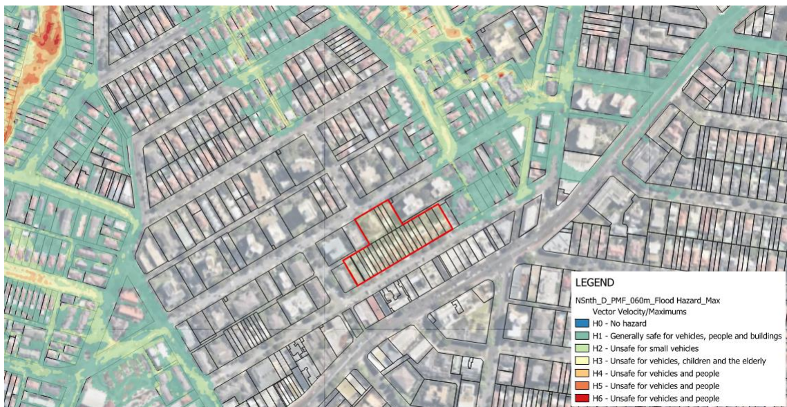
Figure 24 – Maximum flood hazard for 1 hour duration rainfall – PMF (post-developed conditions)
