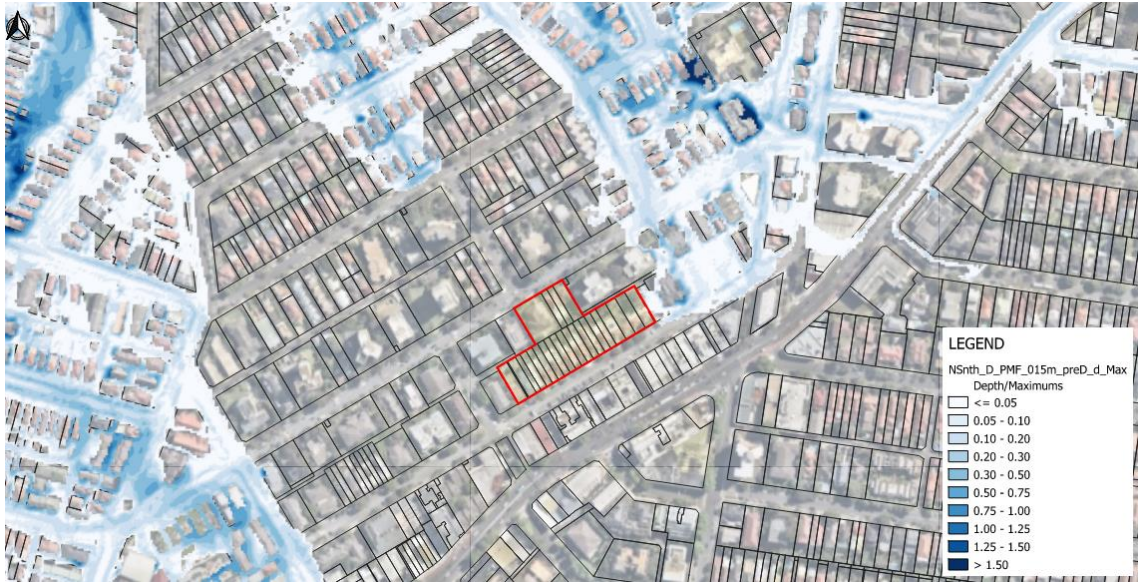
Figure 10 – Maximum flood depth for 15 minutes duration rainfall – PMF (pre-developed conditions)
