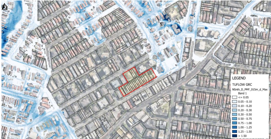
Figure 7 – Maximum depth for 15 minutes duration rainfall – PMF (GRC, 2022)
