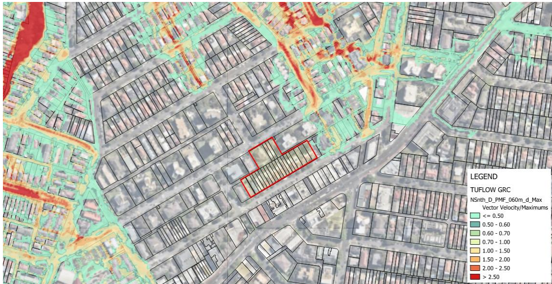
Figure 14 – Maximum velocity for 1 hour duration rainfall – PMF (pre-developed conditions)
