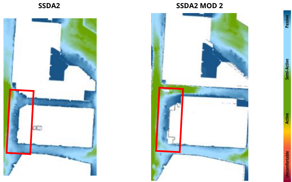
Image 2C: Comparison of Wind Conditions at Ground Level Residential Lobby Entrance for SSDA2 and SSDA2 MOD 2 Designs
