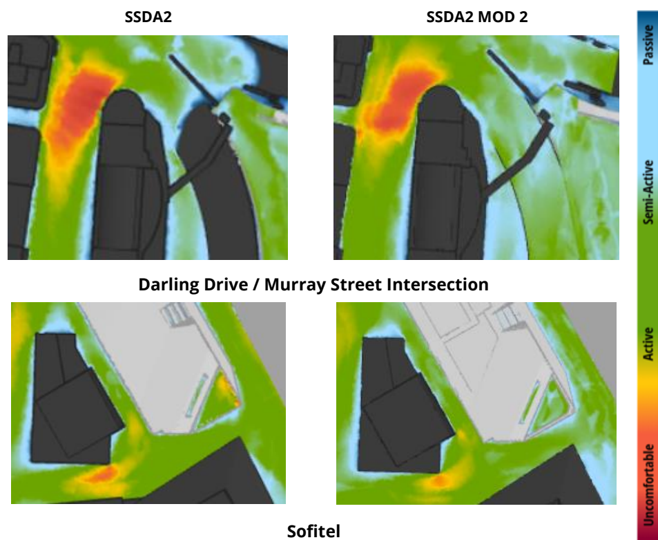
Image 2A: Comparison of Wind Conditions on Ground Level for SSDA2 and SSDA2 MOD 2 Designs
