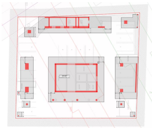
Figure 43 Preliminary shallow pad foundation solution for basement
