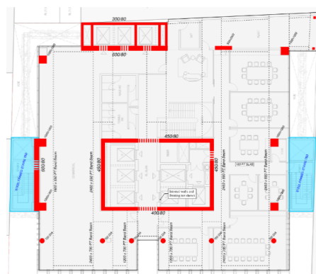
Picture 36 Structural solution for commercial levels
