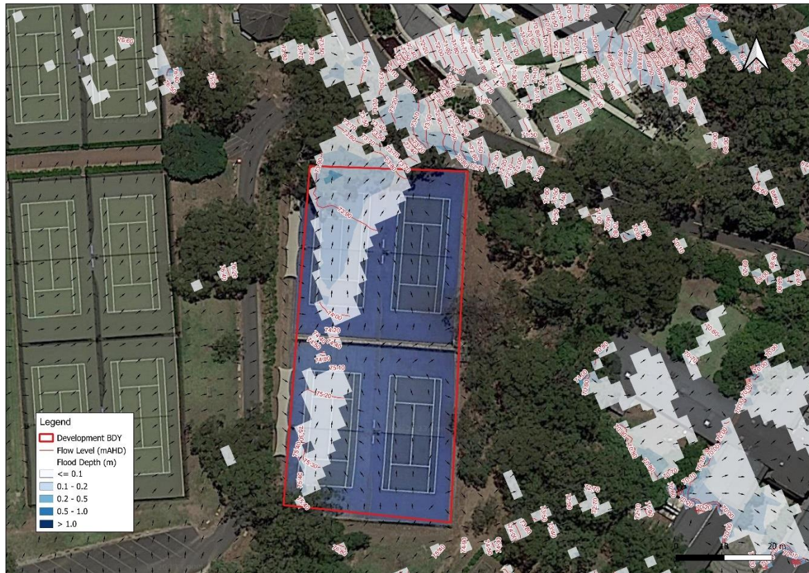
Figure 6 : Existing 1% AEP Flow Depths and levels
