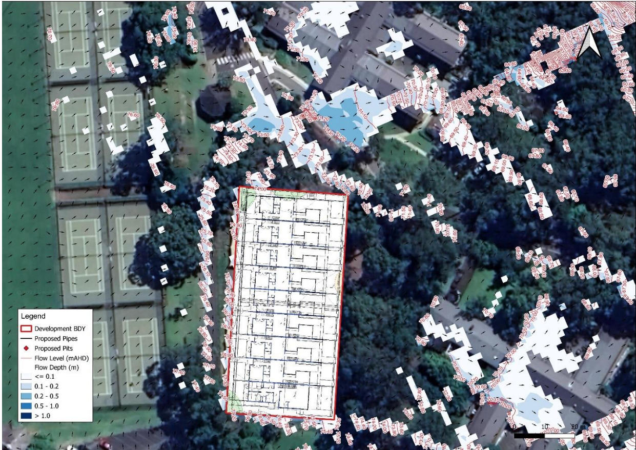
Figure 26- Post Development 1% AEP Flow depths and levels
