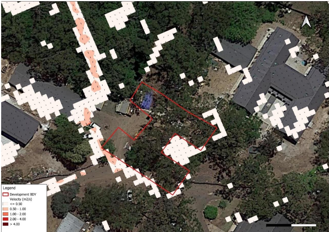
Figure 33: Post Development 1% AEP Flow velocities
