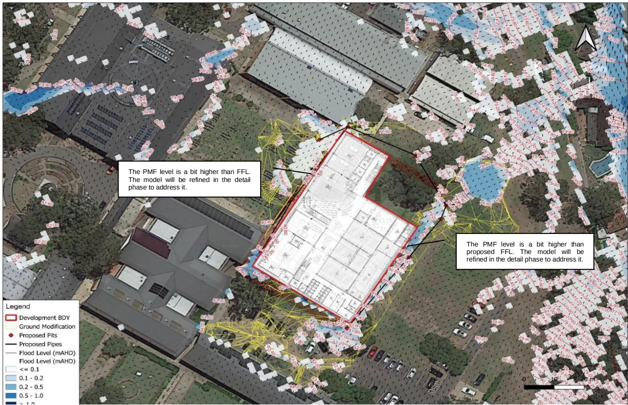
Figure 16: Post Development PMF Flow depths and Levels for Site1
