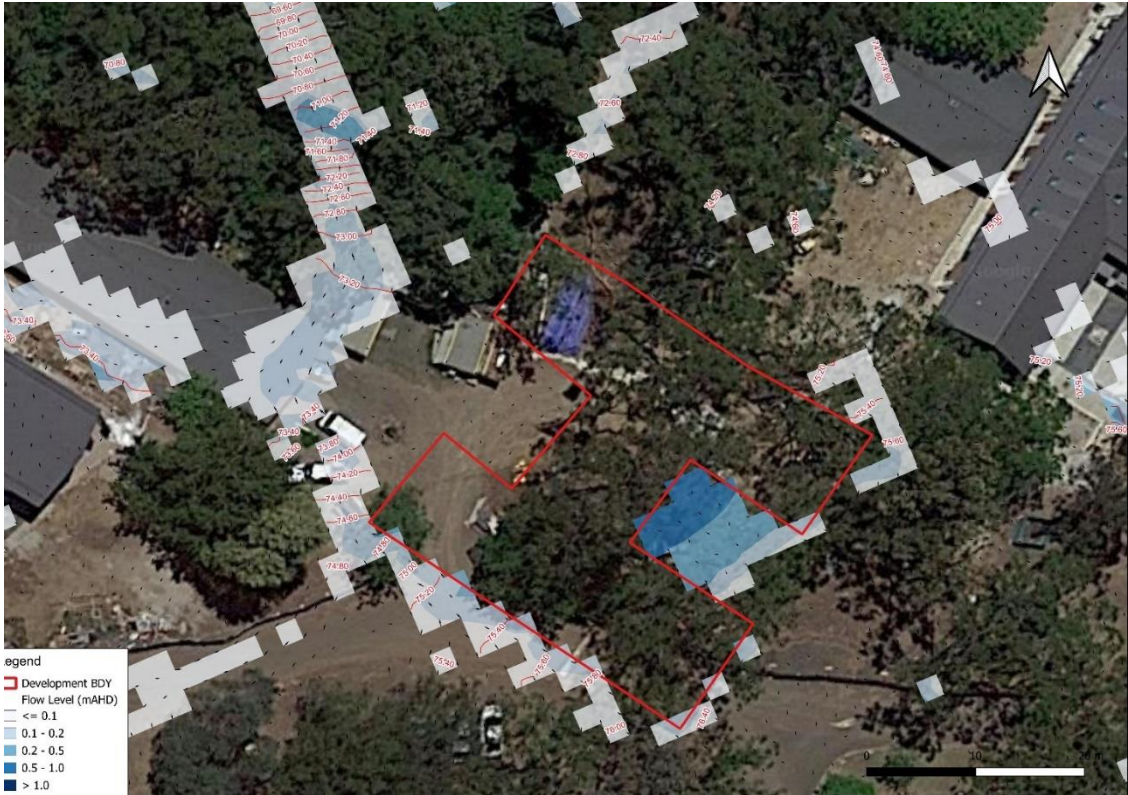
Figure 32: Post Development 1% AEP Flow depths and levels
