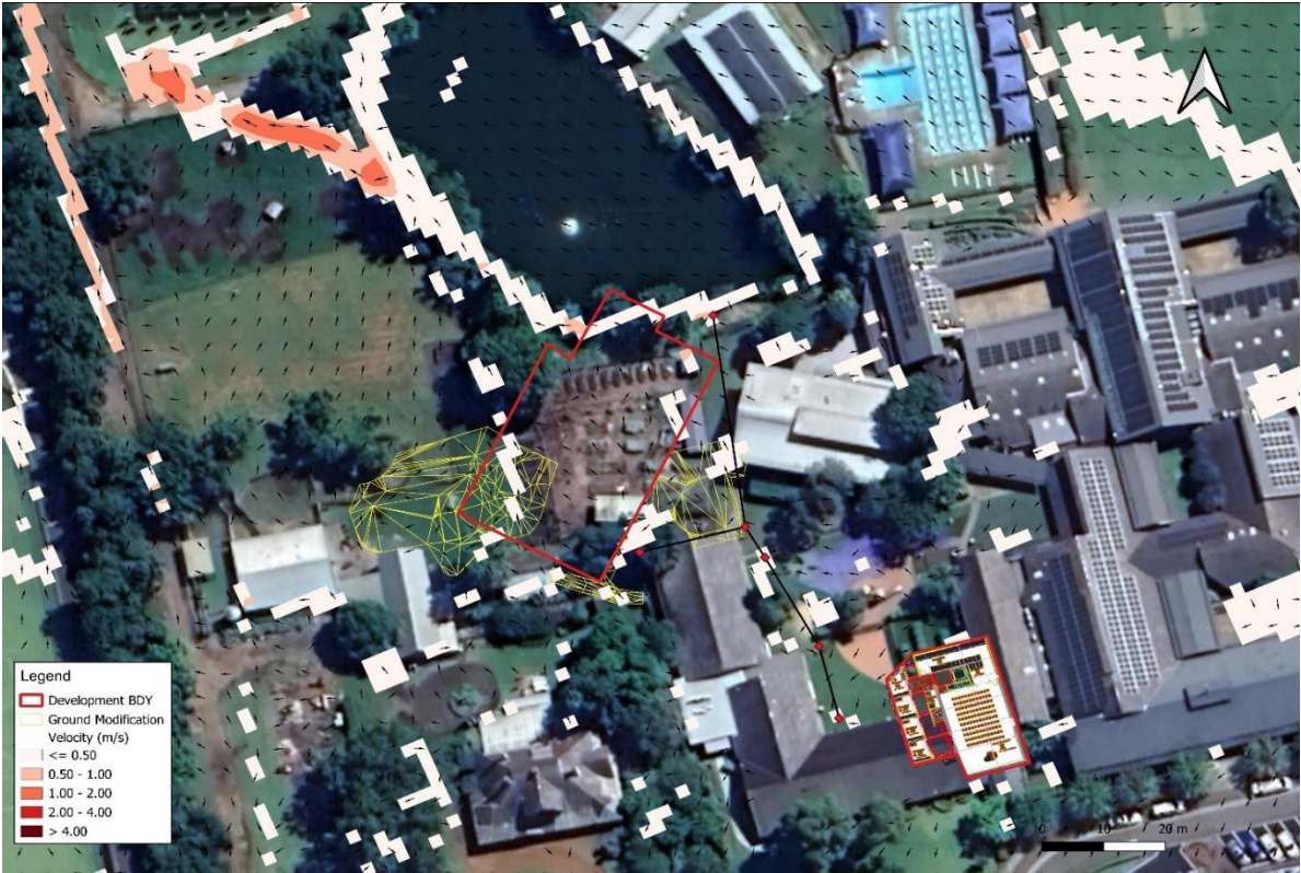
Figure 21: Post Development 1% AEP Flow Velocity
