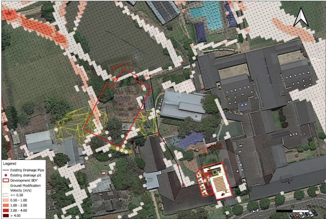
Figure 24: Post Development PMF Flow velocity
