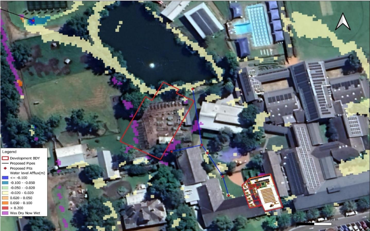
Figure 46- Post Development Afflux (change in flood level) - 1% AEP Storm Event for Site 2A and 2B
