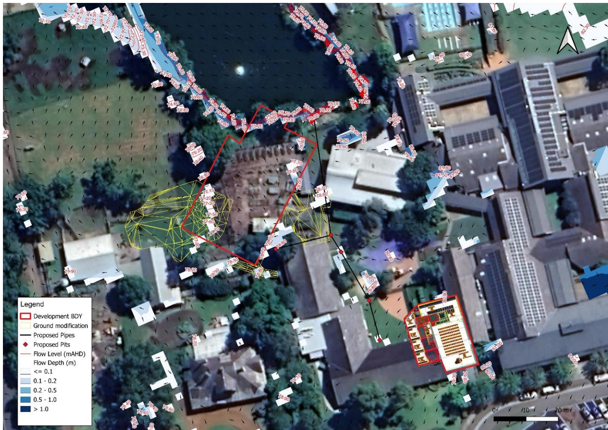
Figure 20: Post Development 1% AEP Flow depths and levels
