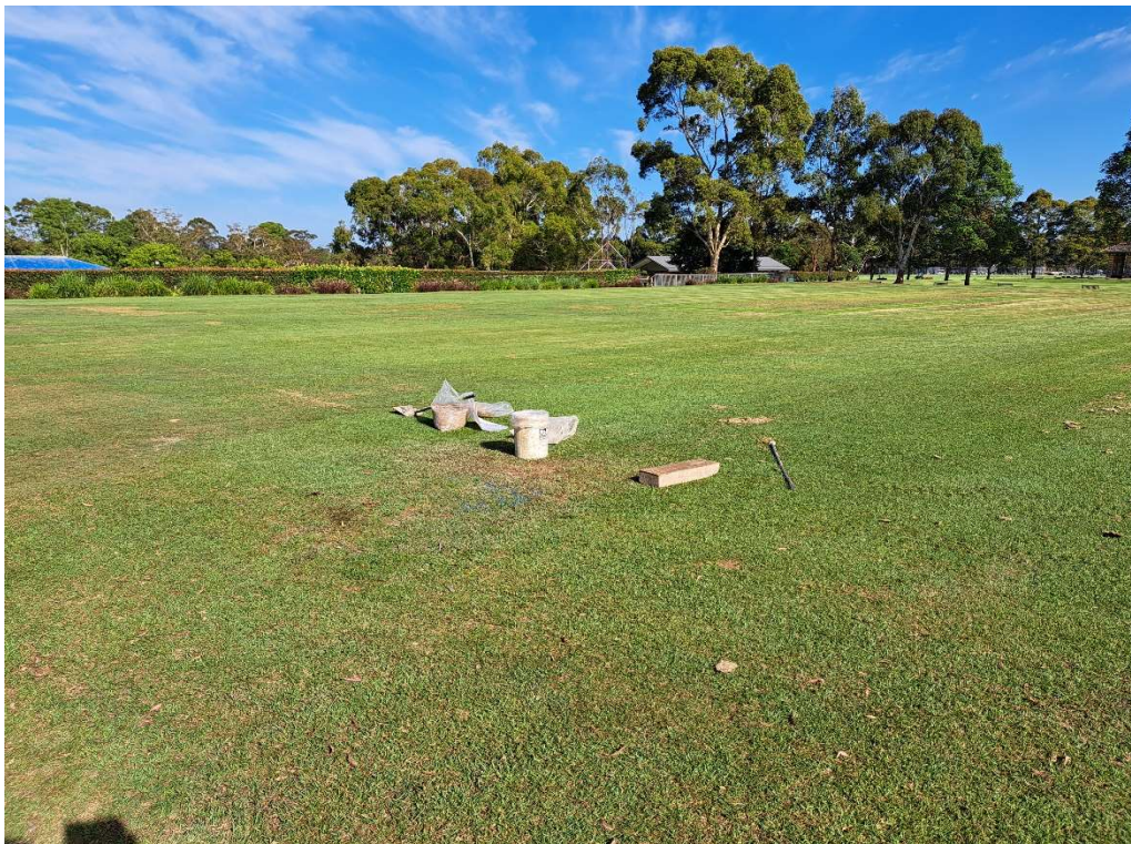
Photo 16 - Typical reinstated borehole (BH07)
