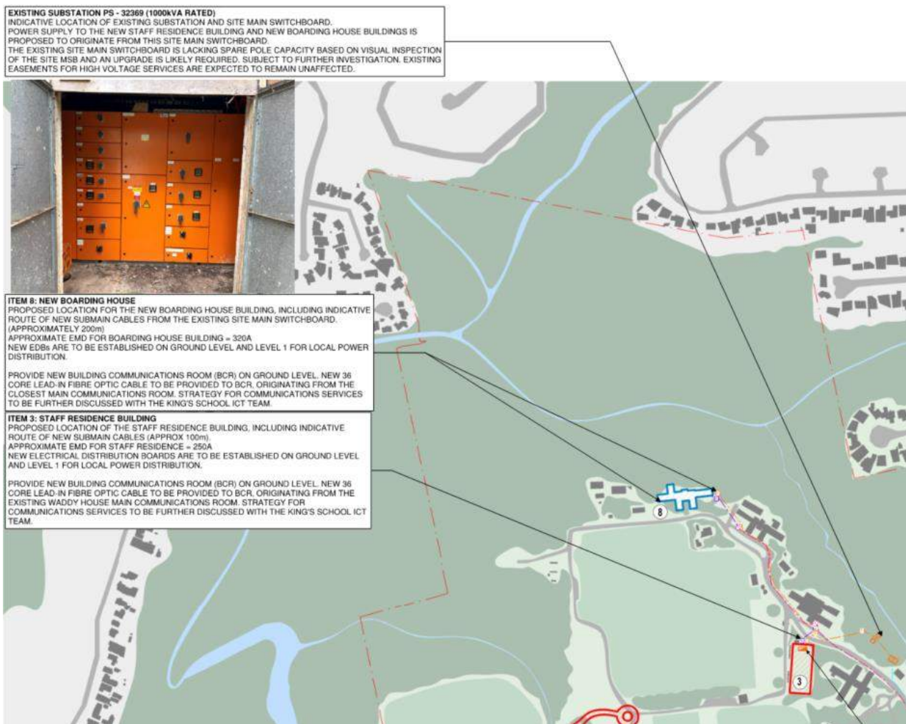
FIGURE 6: BOARDING HOUSE ELECTRICAL INFRASTRUCTURE SITE PLAN
