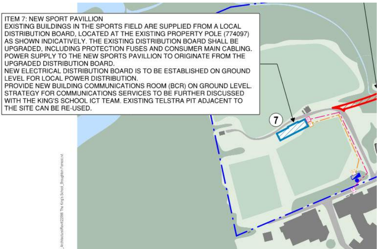
FIGURE 5: SPORTS PAVILLION ELECTRICAL INFRASTRUCTURE SITE PLAN
