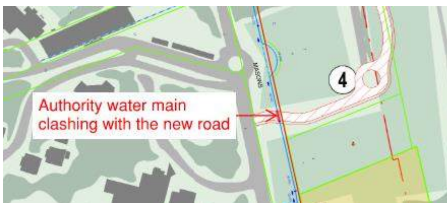
FIGURE 2 THE SECTION OF THE SYDNEY WATER POTABLE COLD-WATER MAIN THAT CLASHES WITH THE NEW ROAD.
