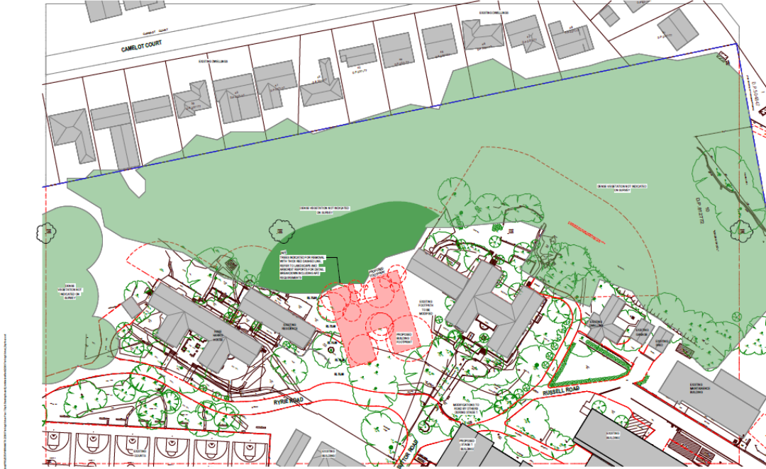
Figure 9 – Demolition Plan to facilitate the proposed concept and envelope of the new day boy house.
