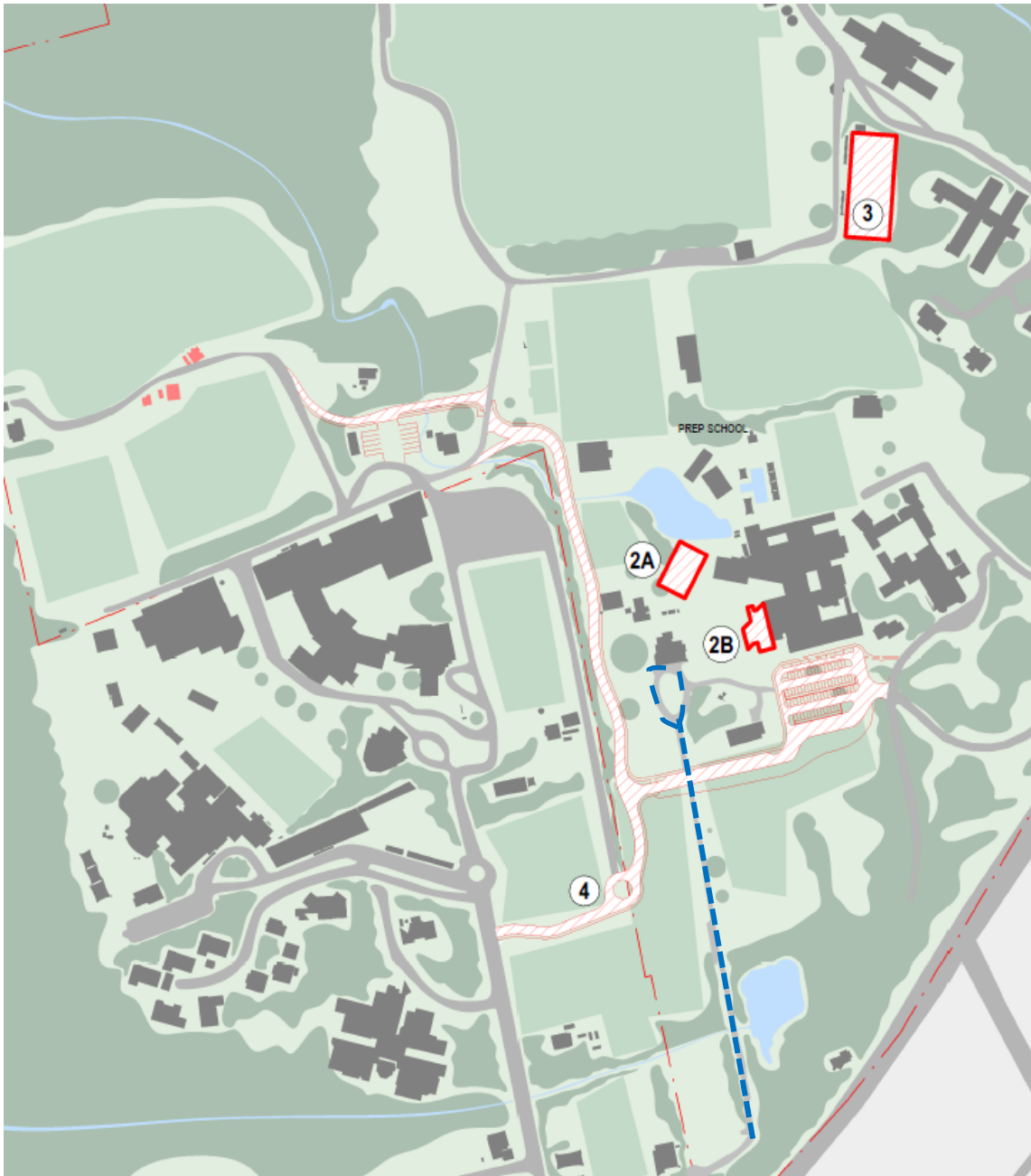
Figure 128 – Part plan showing the proposed new access road and parking in front of the Prep School. The original driveway to Cedars and carriage loop are indicated by the blue dashed line
