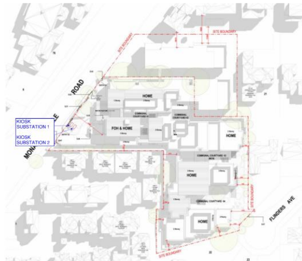
Proposed Substation Location - Site Plan
