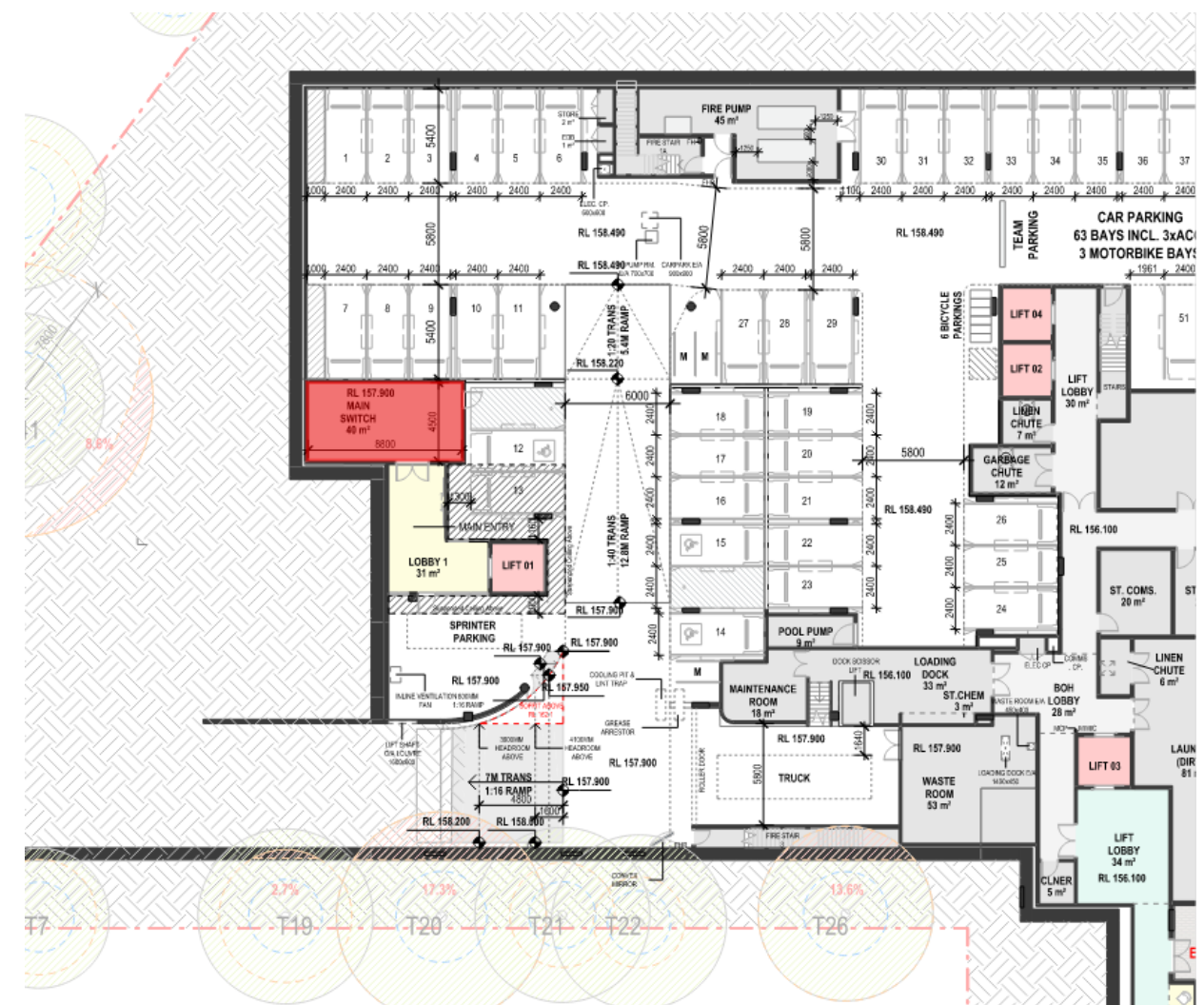
Proposed Switch Room Location On Ground Floor
