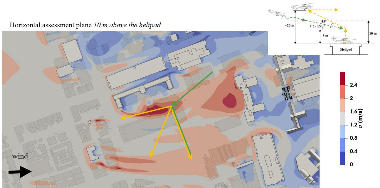
Figure 35: Wind induced turbulence in a horizontal plane 10 m above the helipad for the wind from west.
