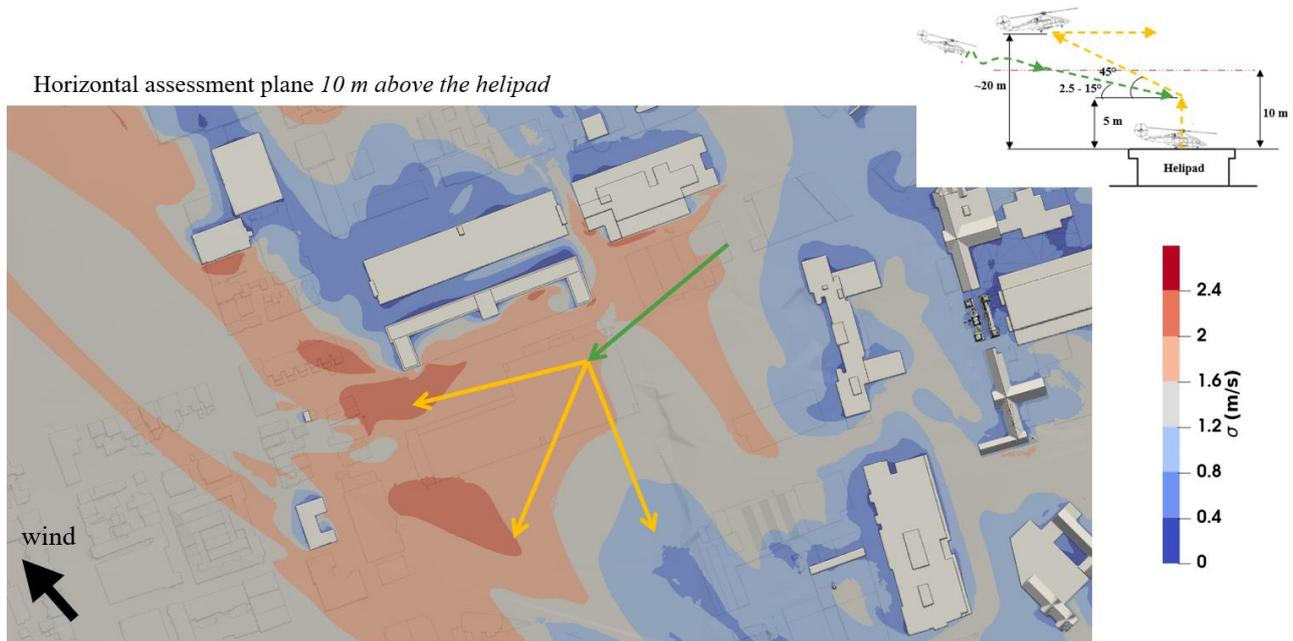
Figure 33: Wind induced turbulence in a horizontal plane 10 m above the helipad for the wind from south-east.
