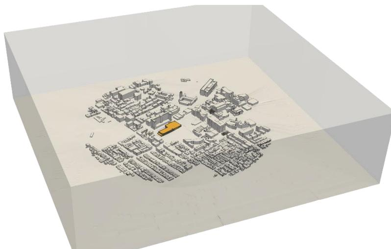
**Figure 9. Simulation domain based on the dimension of the tallest building modelled.**
