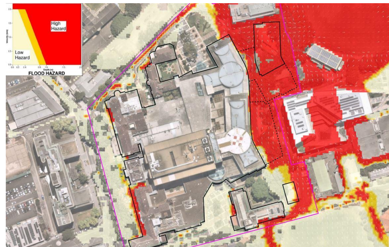
Figure 14 – East Campus post-development PMF Hydraulic Hazard
