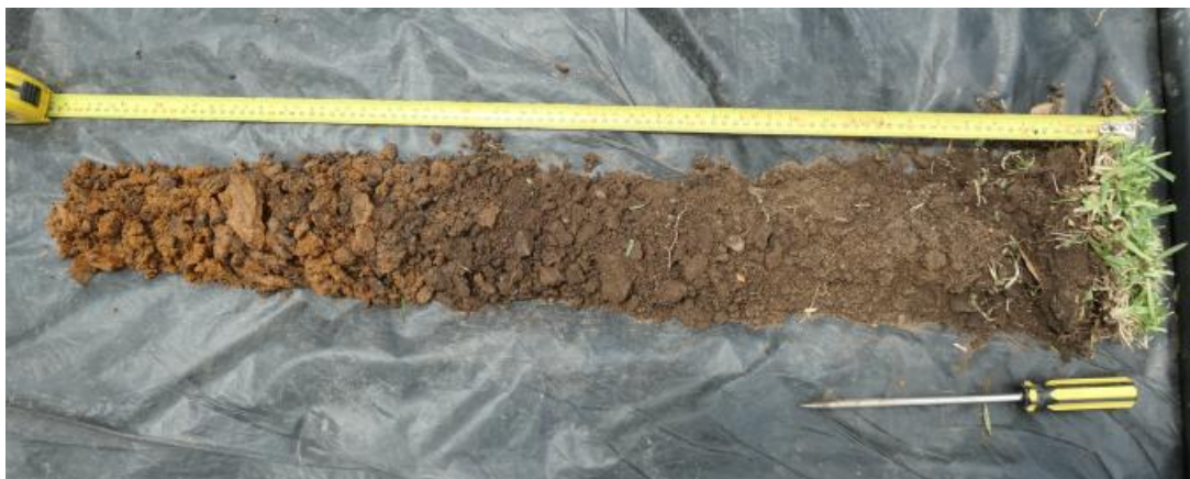
Figure 2.5 – Soil sample with clay loam soil to 400mm then very heavy clay below this. (Photo: Arterra 22/12/21)
