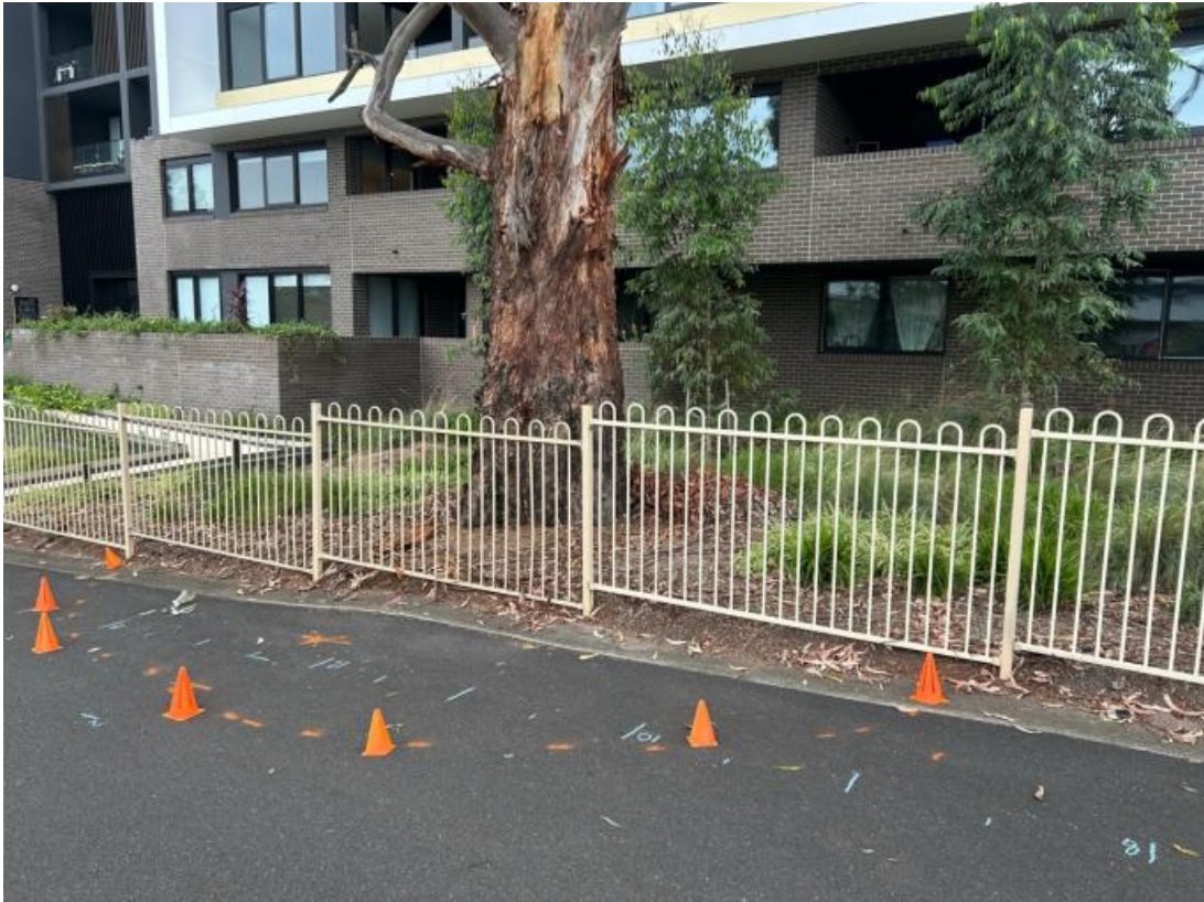
Figure 2 – Image of the area where GPR root investigations were carried out. The SRZ of the tree was clearly defined with the witches hats and spray paint. Note the recently completed gardens and new Euc. saligna planting. (Photo: Arterra 1 March 2024)
