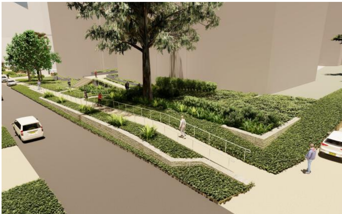
Figure 2.15 –Illustrative render of proposed design highlighting the implementation of a retaining wall to maintain the existing levels to the north of the tree (Illustrative Render: Arterra)
