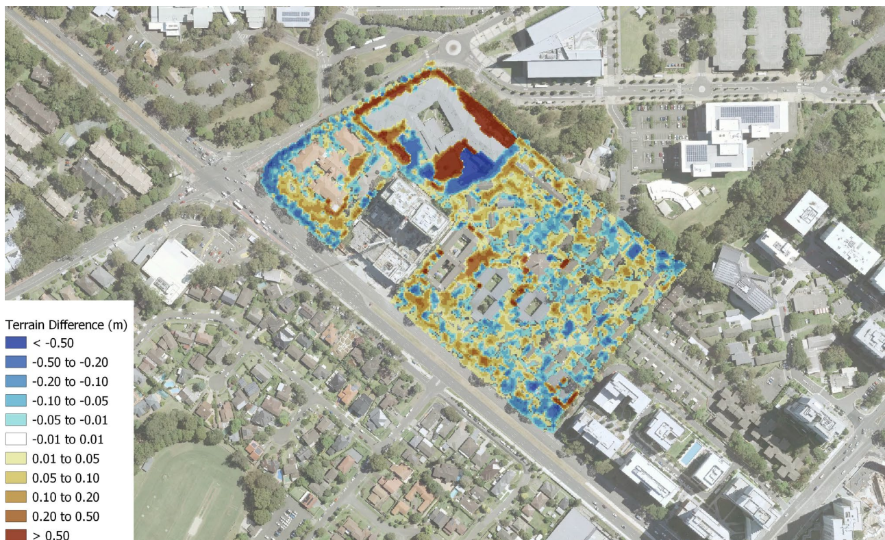
Figure 8 Ground Level Differences (m) (Survey – LiDAR Levels)
