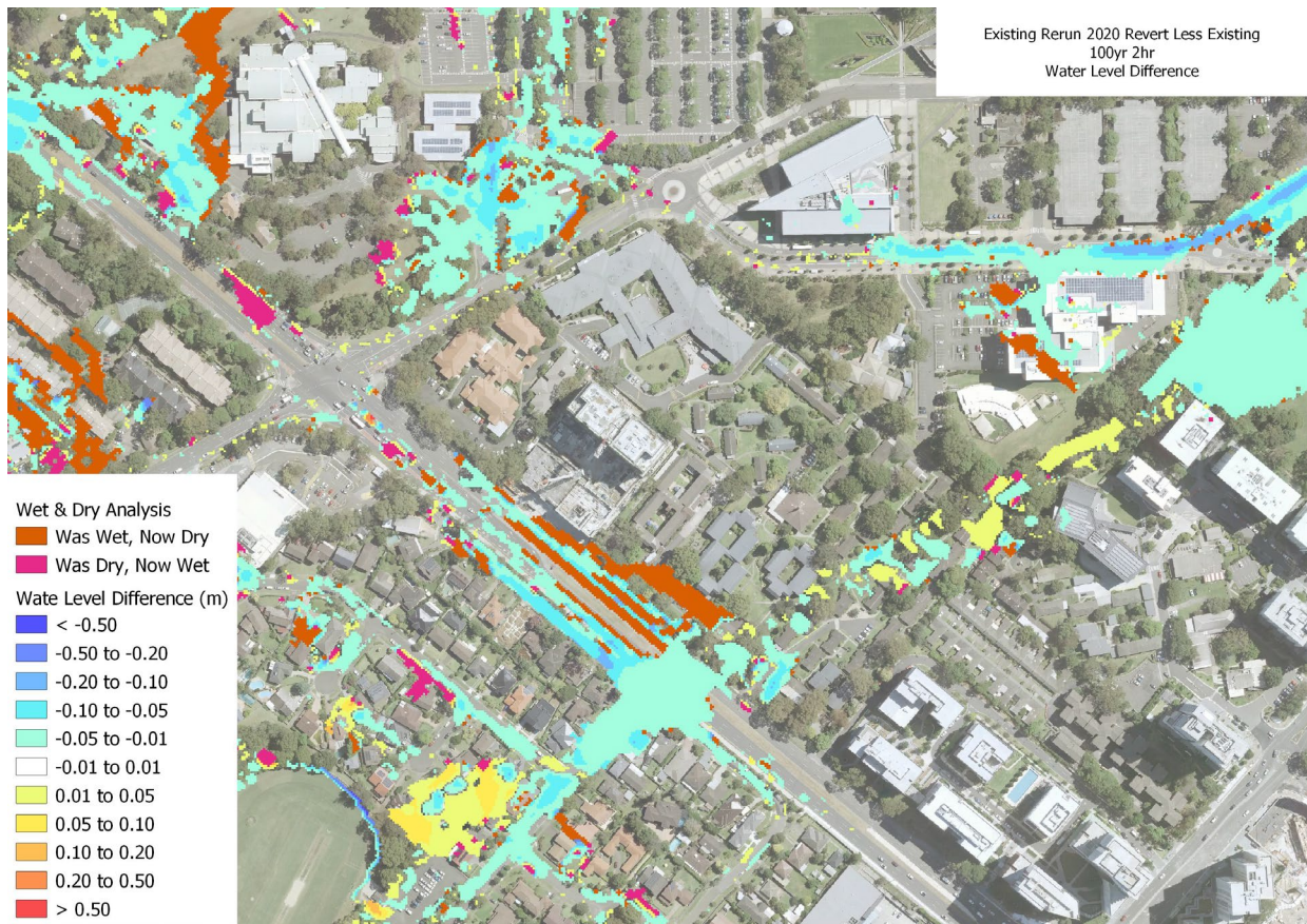
Figure 12 100 yr ARI Flood Level Differences (2020 TUFLOW – 2008 TUFLOW runs)
