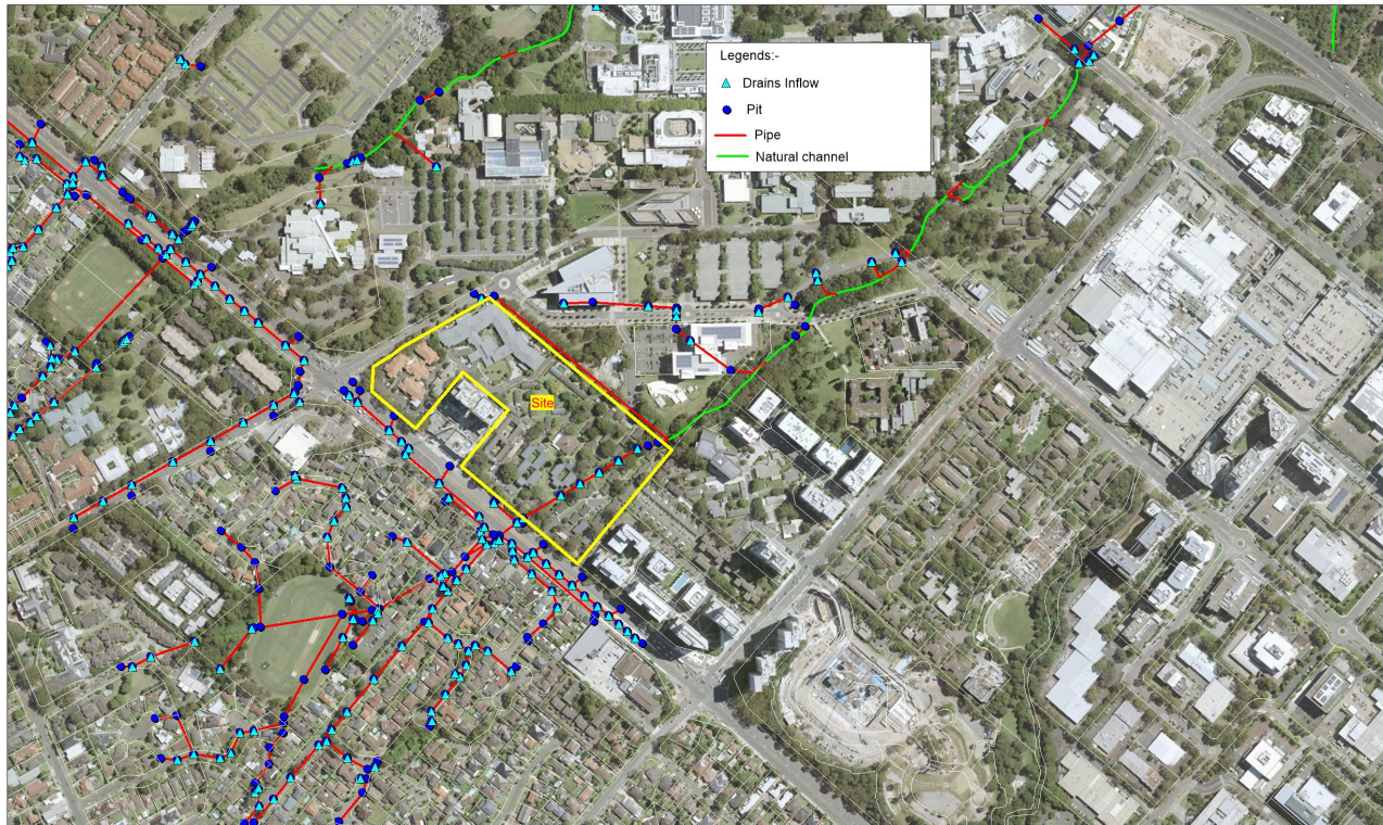
Figure 10 View of DRAINS Model Inflows in University Creek Catchment
