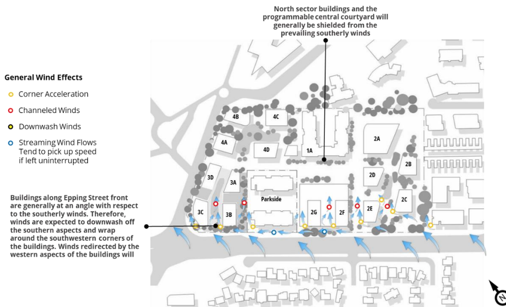
Figure 6: Expected Wind Flow Patterns within the Proposed Masterplan due to Southerly Sector Winds
