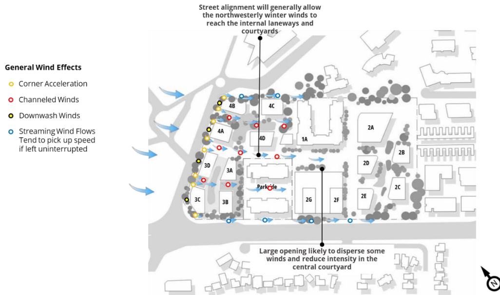
Figure 9: Expected Wind Flow Patterns within the Proposed Masterplan due to Northwestern Sector Winds
