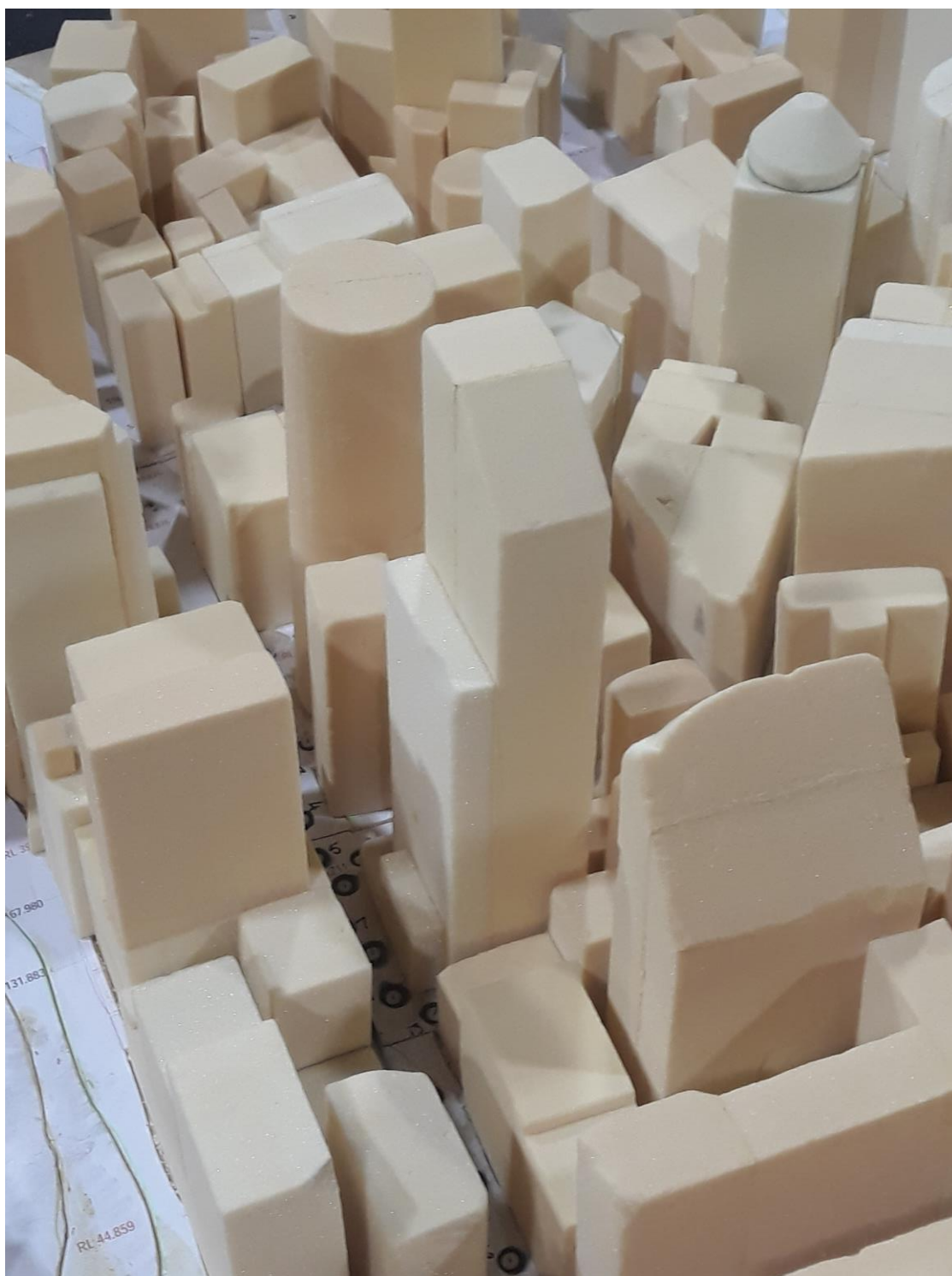
Figure 3-6 Wind tunnel model showing the proposed development
