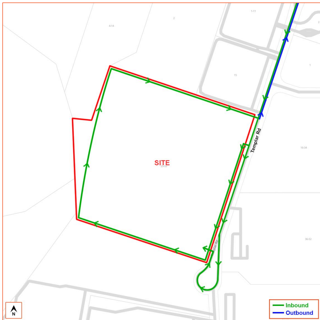
Figure 4: Truck Access and Internal Circulation (Illustrative)
