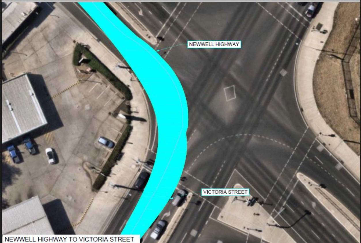
NEWWELL HIGHWAY TO VICTORIA STREET LHT MITCHELL HWY FROM NEWELL HWY (SWEPT PATH)
