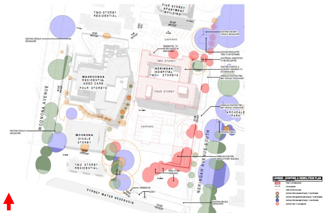
Figure 57: Existing and demolition site plan. (Source: Bickerton Masters Architects)
