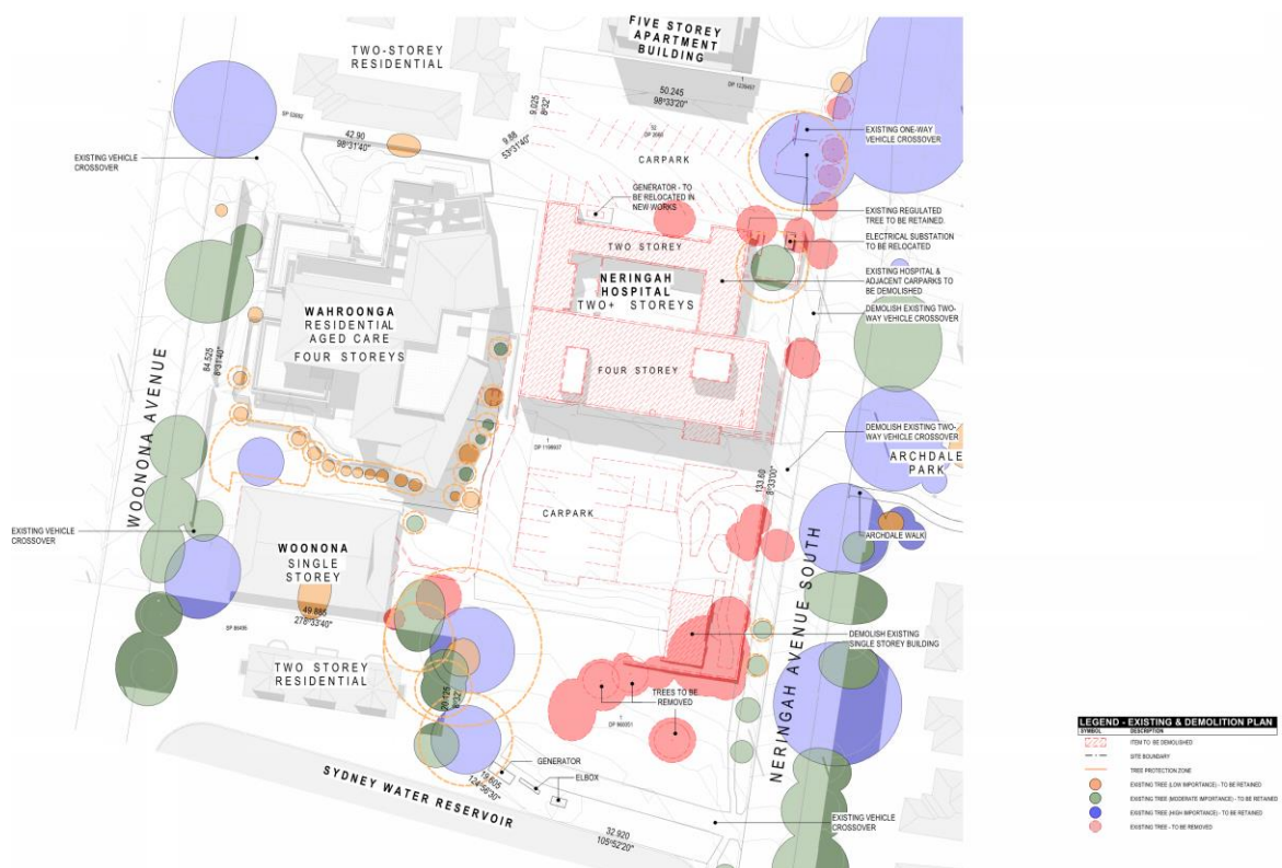
Figure 2 Existing Site Layout & Proposed Demolition Plan
