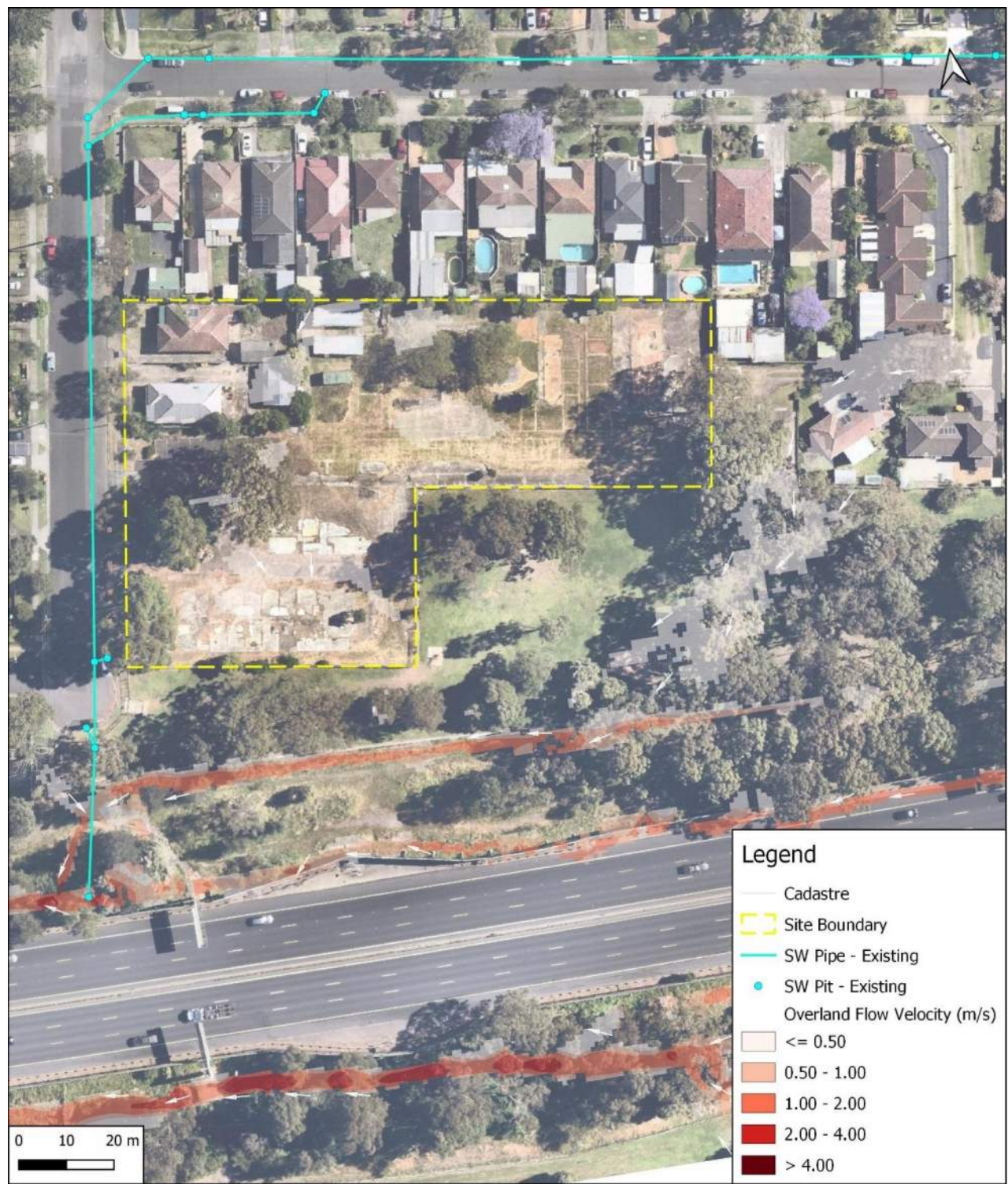
Figure 5 - 1%AEP Overland Flow Velocity – Existing Conditions
