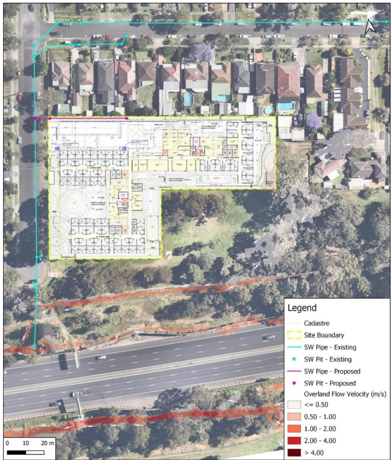
Figure 11 - 1%AEP Overland Flow Velocity – Proposed Conditions
