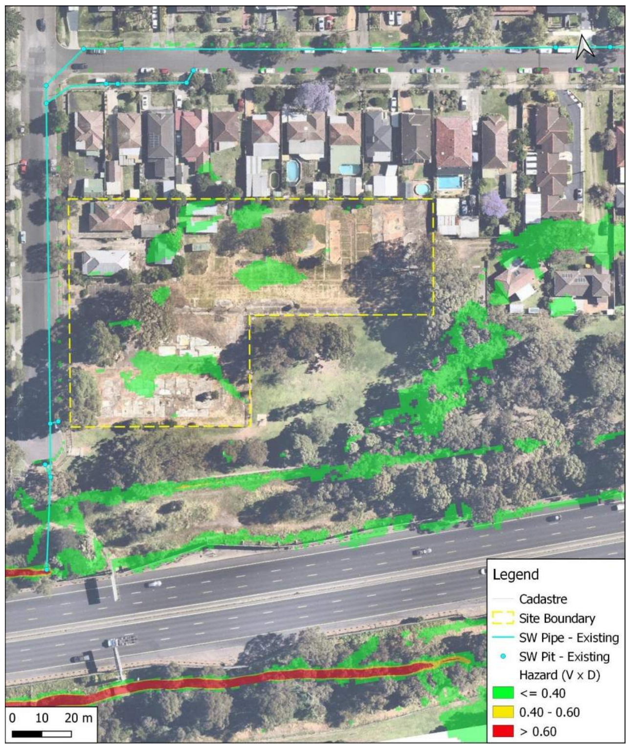
Figure 6 - 1%AEP Overland Flow Hazard – Existing Conditions
