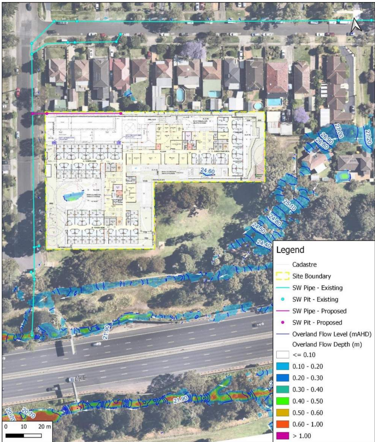
Figure 10 - 1% AEP Overland Flow Level & Depth – Proposed Conditions
