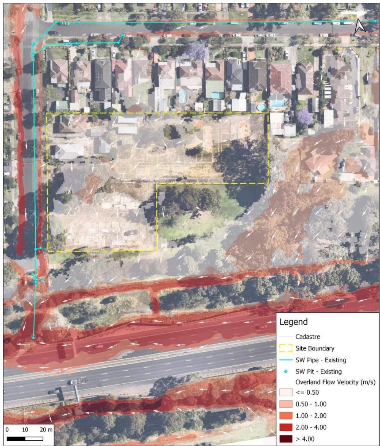
Figure 8 PMF Velocity – Existing Conditions
