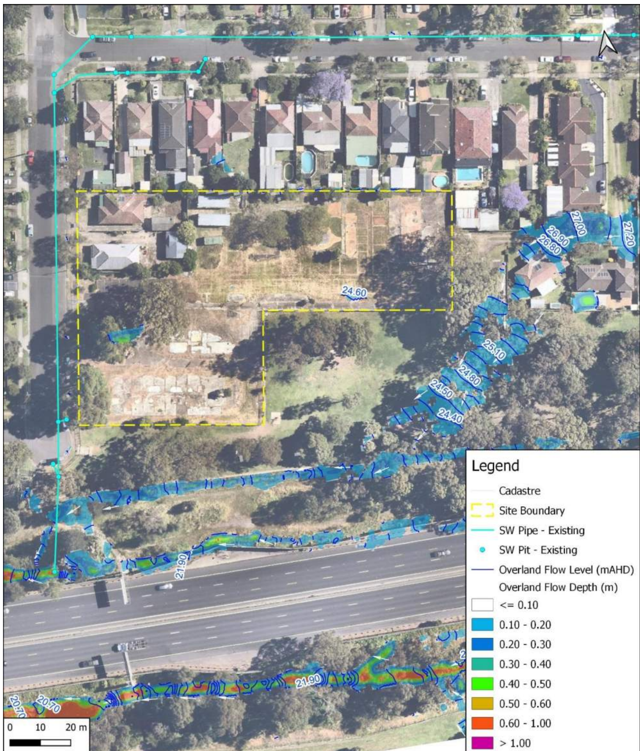
Figure 4 - 1%AEP Overland Flow Level & Depth – Existing Conditions
