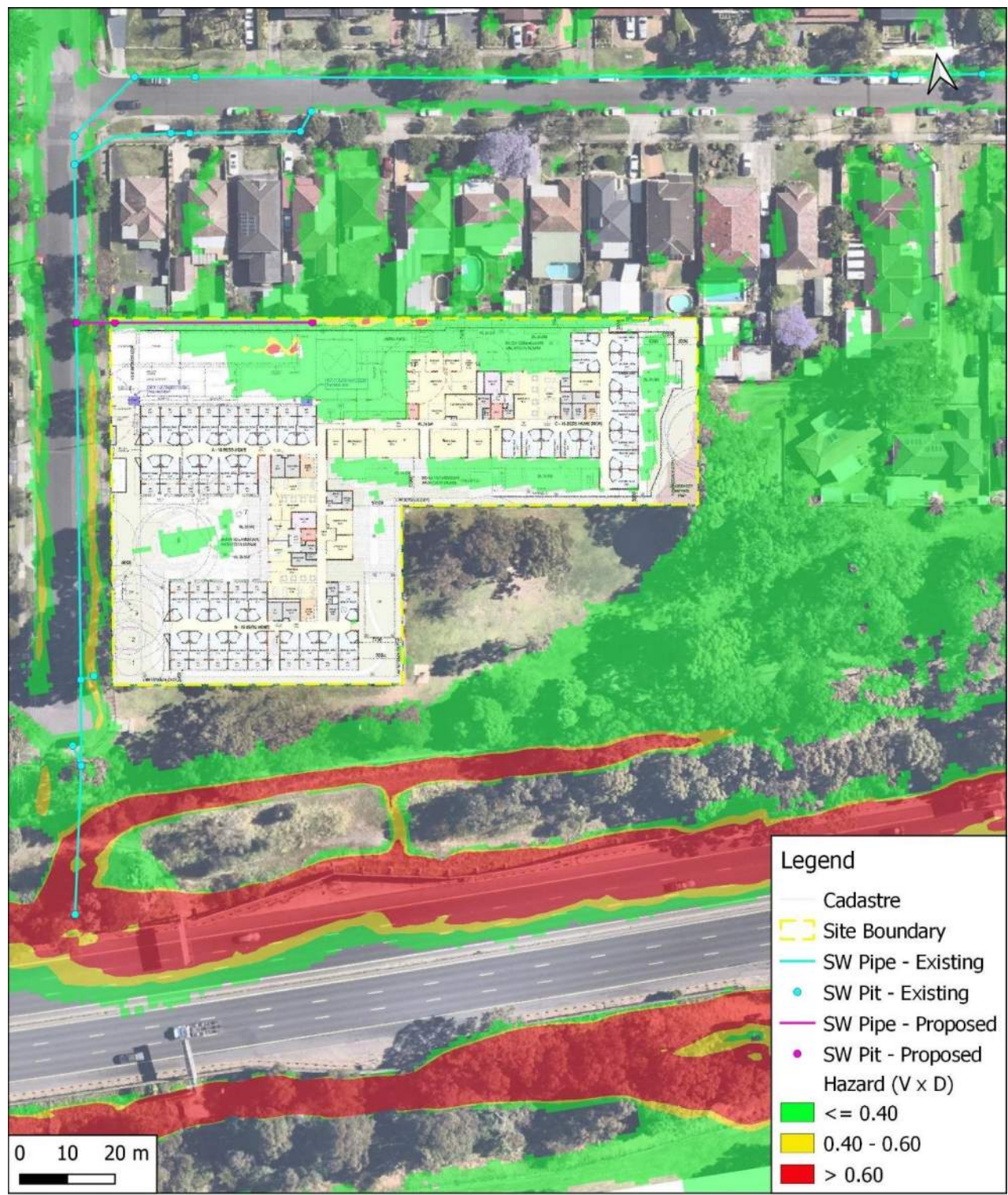
Figure 15 - PMF Hazard – Proposed Conditions
