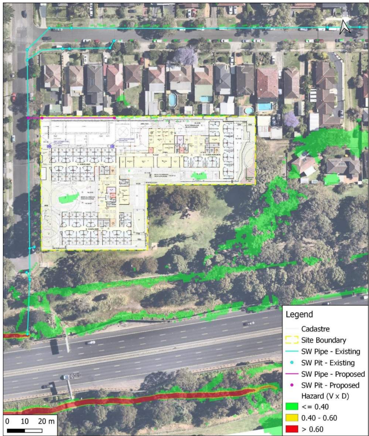
Figure 12 - 1%AEP Overland Flow Hazard – Proposed Conditions
