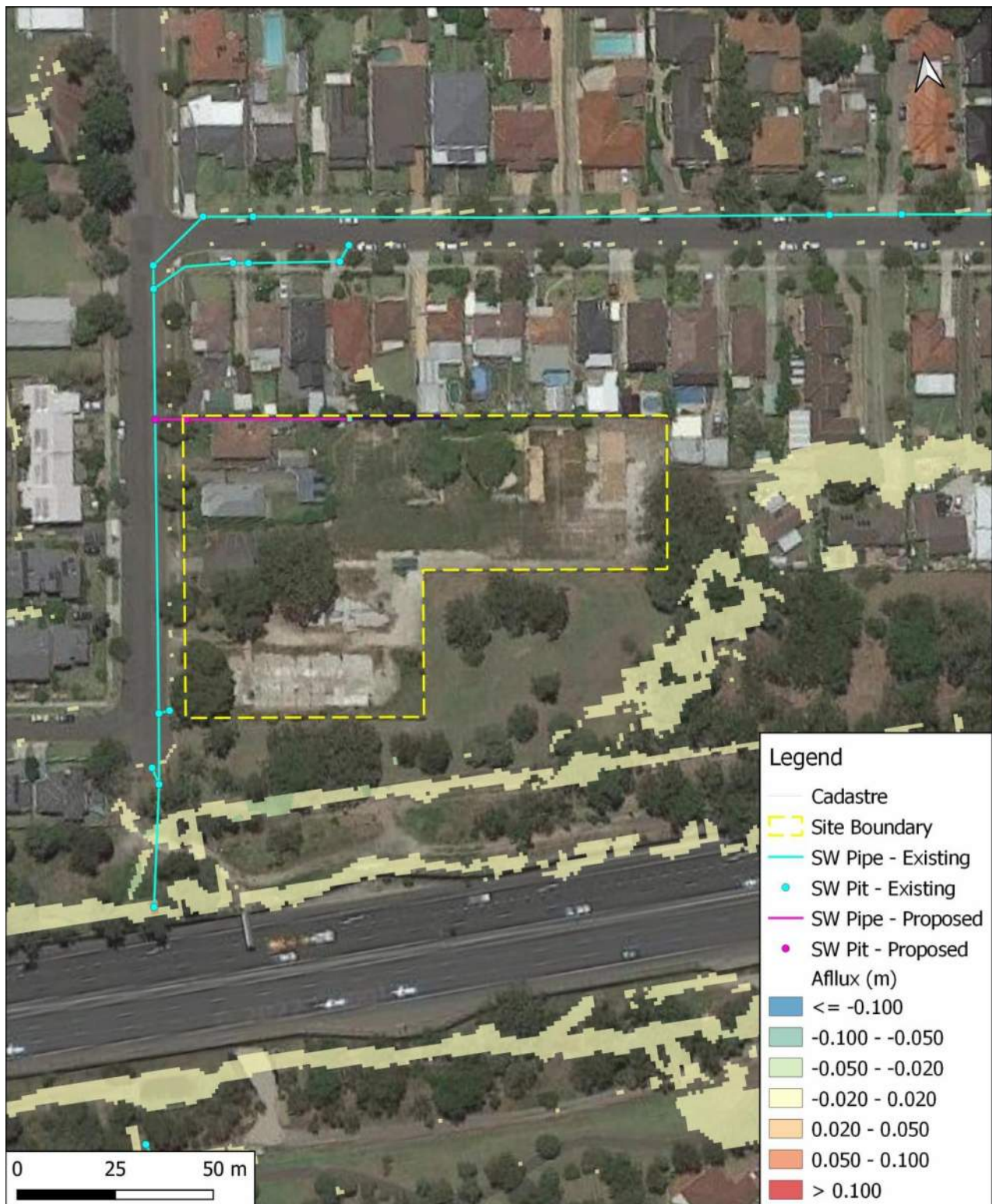
Figure 16 - 1%AEP Flood Level Impacts– Proposed Conditions
