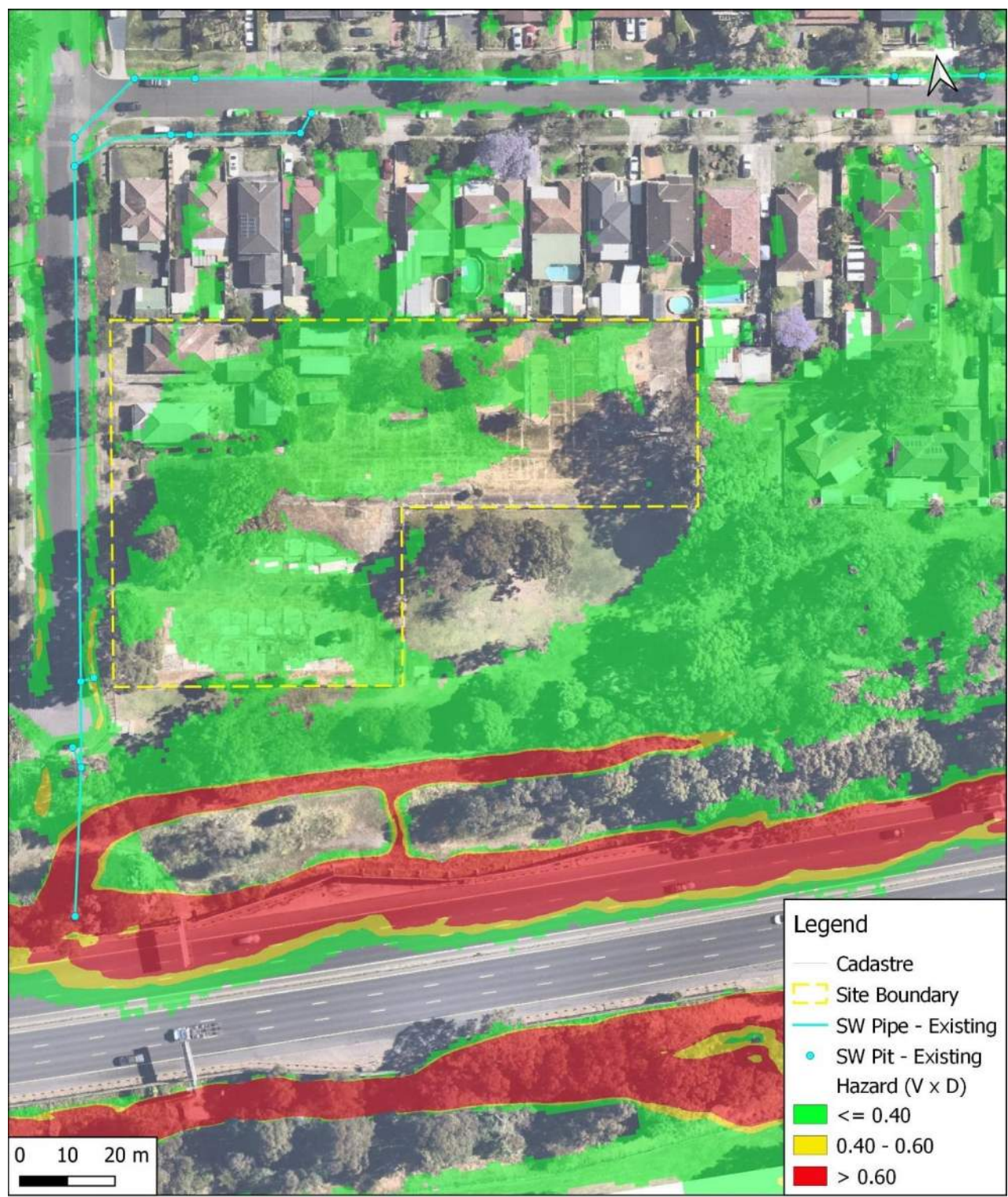
Figure 9 - PMF Hazard – Existing Conditions
