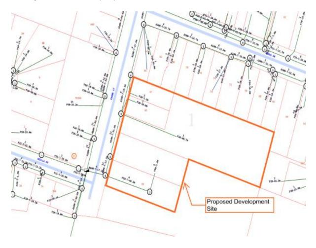
Jemena Assets – Unencumbered other than disconnections. Area serviced by natural gas mains with 110mm diameter 7kpa low pressure line, located in Karne Street about 17m from the western boundary.
