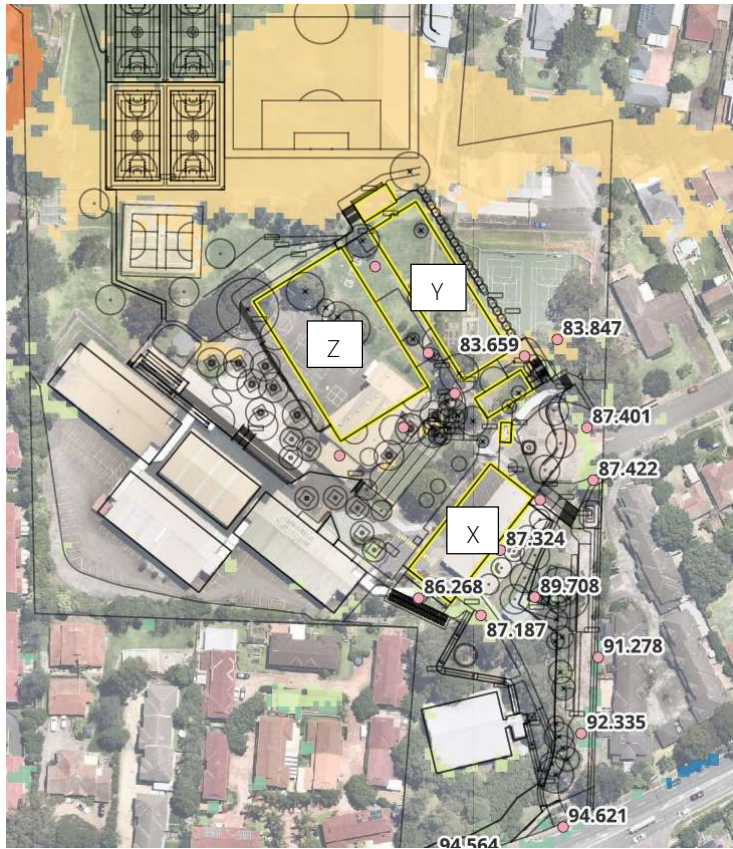
Figure 5 – 1% AEP Levels and Extents for CHS site.
